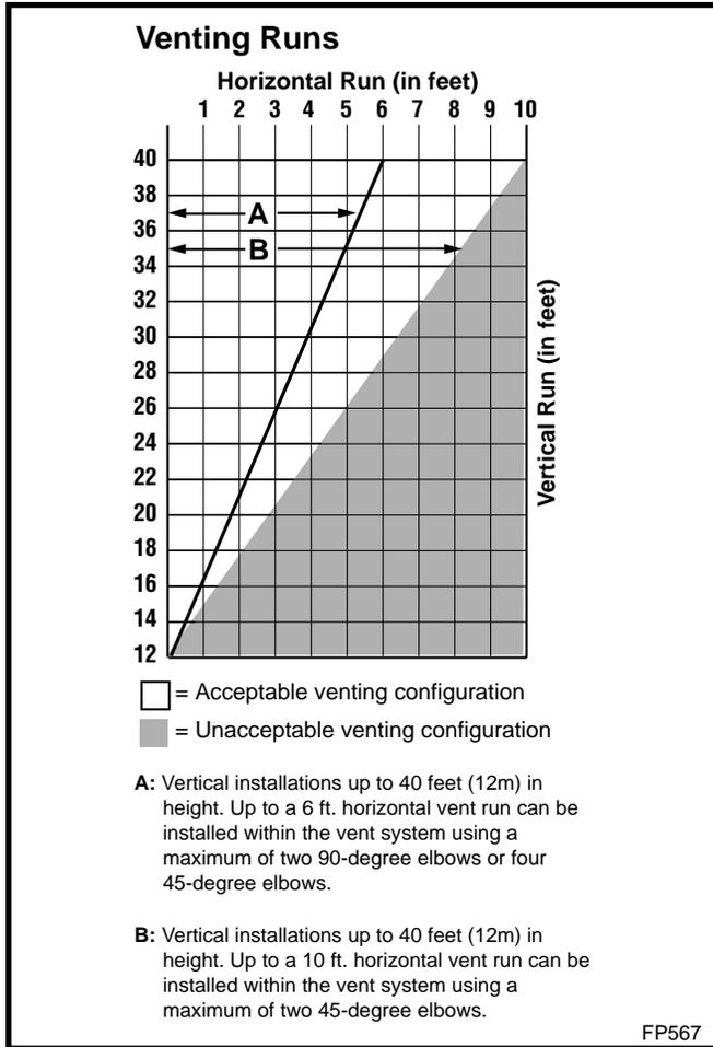
Fig. 13 Venting configurations.
