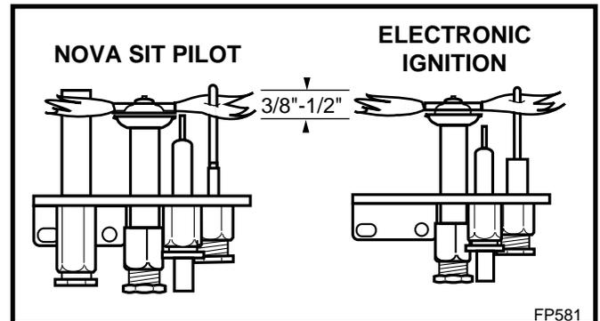
Fig. 20 Proper pilot flame height.
