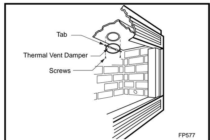
Fig. 21 Attach the thermal vent damper.
