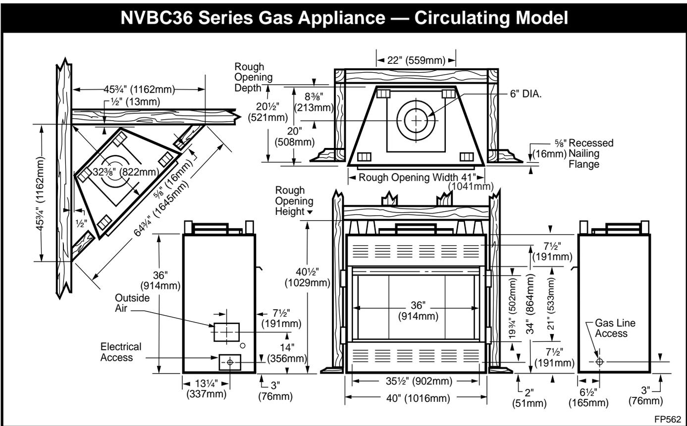
Fig. 2 NVBC36 Series specification and framing dimensions.
