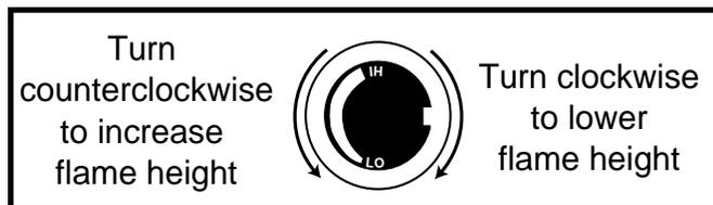
Fig. 17 Flame adjustment knob for SIT820 valve.
