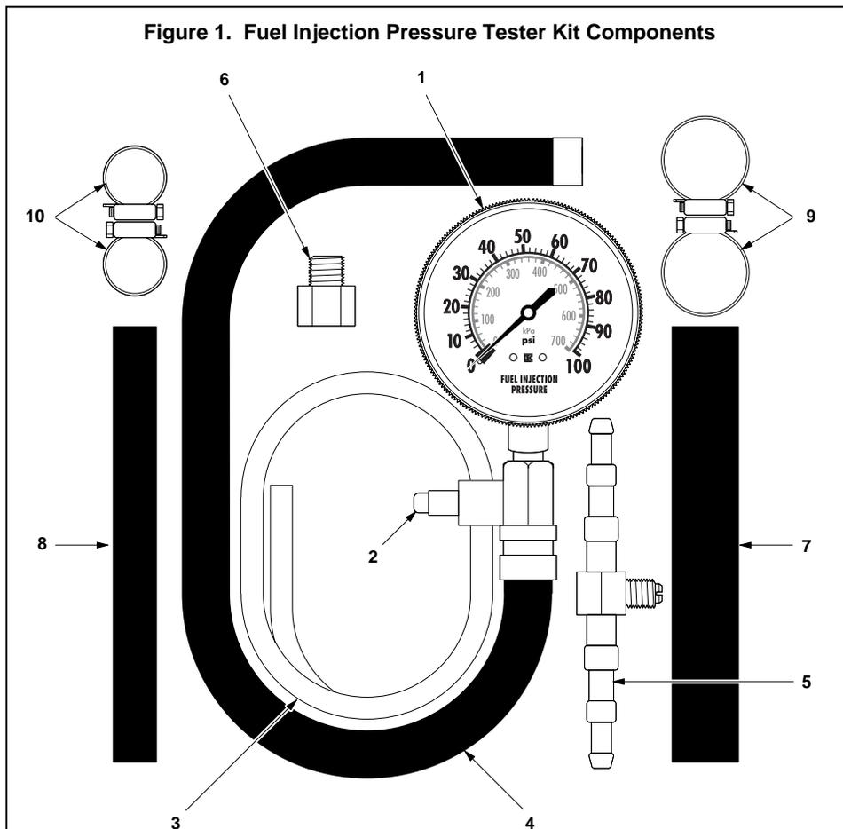
1. **Tester Gauge.** Shows fuel pressure in system during test.
