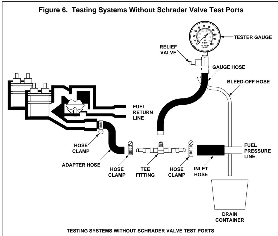
**WARNING:** *Systems without test ports require that fuel lines be removed or disconnected. Please be aware that these lines may be UNDER PRESSURE, and when removed could cause fuel spray and/or leakage onto hot engine parts.*
