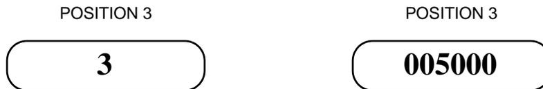
The above example indicates the previously programmed test length for position 3 was 50 minutes.
