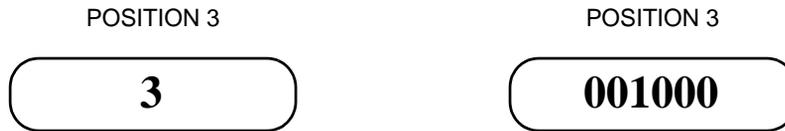
The above example indicates the previously programmed delay time for position 3 was 10 minutes.
