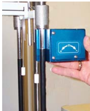
FIGURE 14. Electronic Level Sensor Placement
