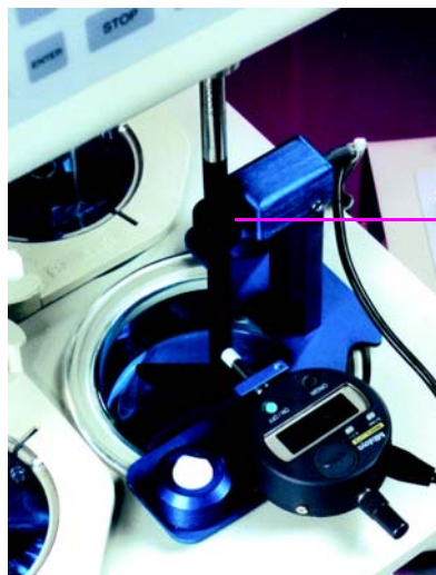
FIGURE 15. Placement for RPM Reading, Paddle
