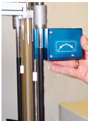
FIGURE 17. Electronic Level Sensor Placement
