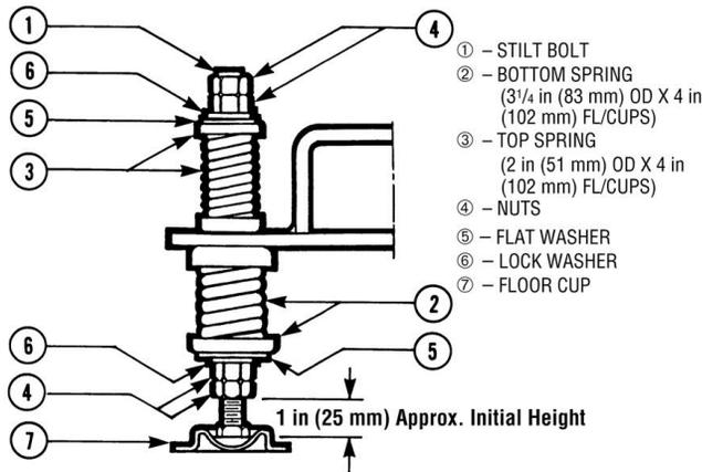
**4.3.3.3 Stilt/spring mounted baseplates - motor alignment (Long-Couple pumps only)**
