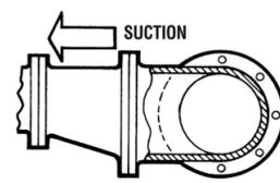
Avoid the use of throttling valves and strainers in the suction line. Start-up strainers must be removed shortly before start up. When the pump is installed below the source of supply, a valve should be installed in the suction line to isolate the pump and permit pump inspection and maintenance. However, never place a valve directly on the suction nozzle of the pump.
