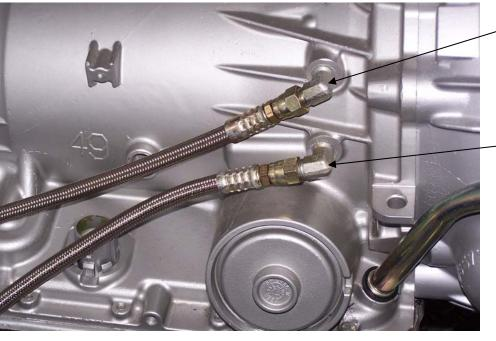
LOWER LINE (OUTLET) – PRESSURE (HOT) LINE TO LOWER RADIATOR/COOLER
