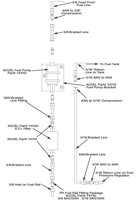
NOTE: If using ACCEL Pump Part #74701, please contact ACCEL/DFI Technical Service for proper plumbing instruction.
