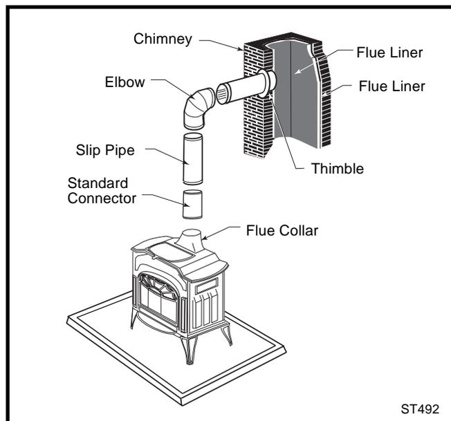
**Fig. 6** Chimney connection is a freestanding installation.
