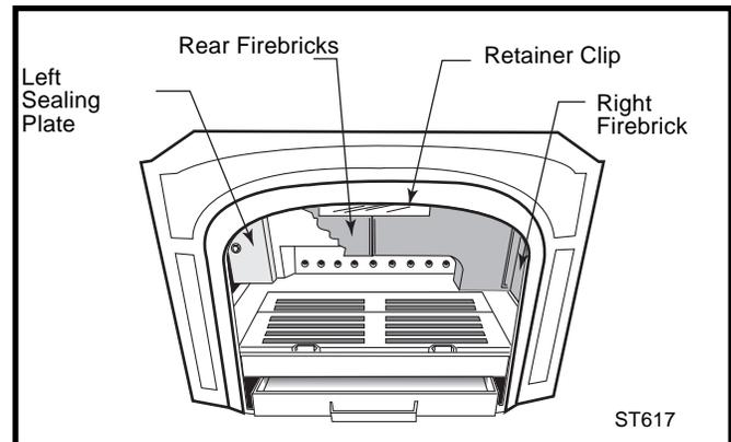
**Fig. 33** Remove left and right sealing plates.
