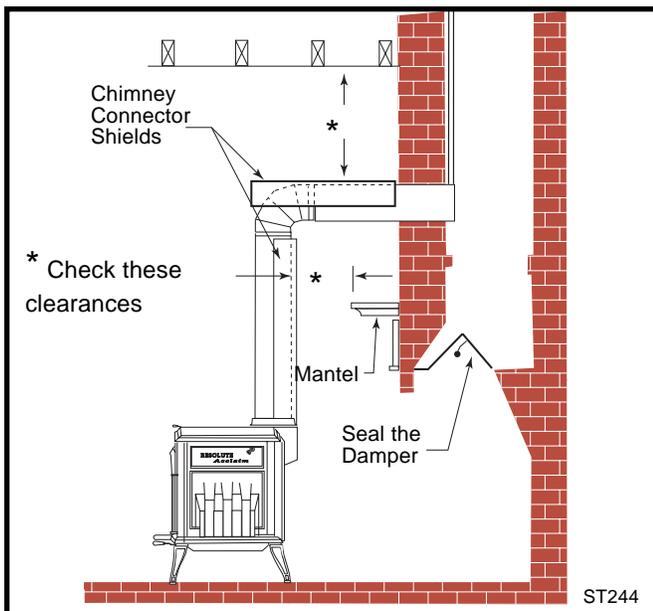
Fig. 7 Chimney connector enters chimney above the fireplace.
