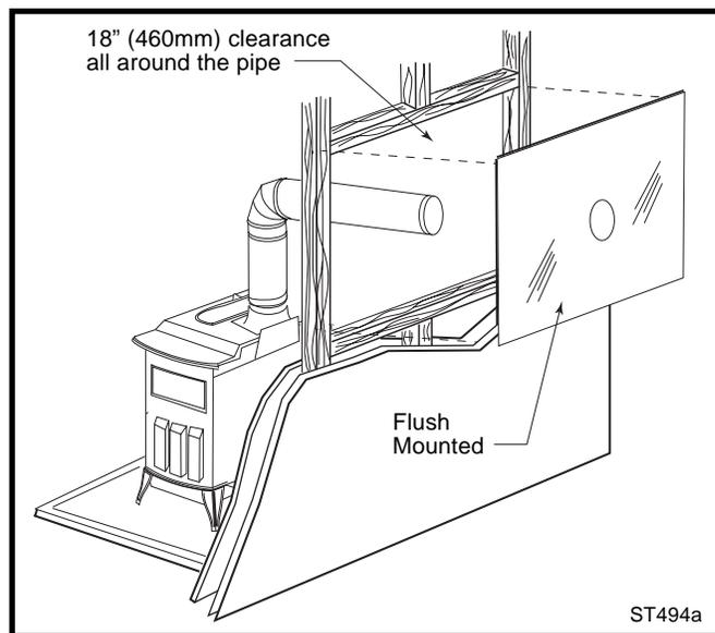
**Fig. 10** An approved wall pass-through for Canada.
