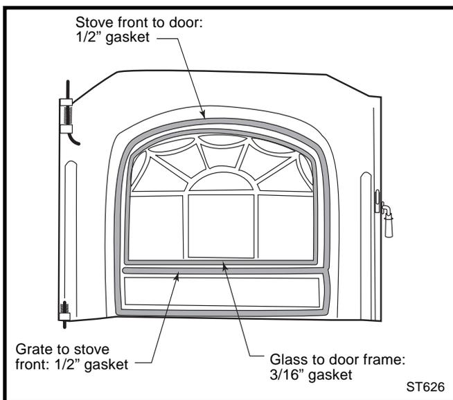
**Fig. 39** Two different gasket sizes are used to seal the front door.
