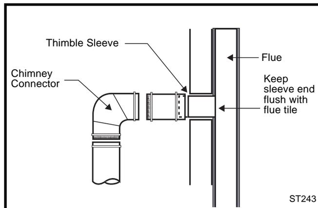
**Fig. 5** The thimble, made of either cermaic or metal, must be cemented securely in place.
