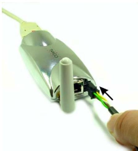
**Figure 13.a:** Connect the DC power supply
