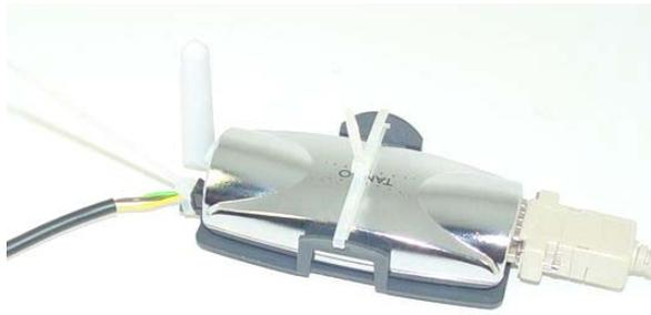
**Figure 14.a** Place the modem on the cradle and firmly fixed.
