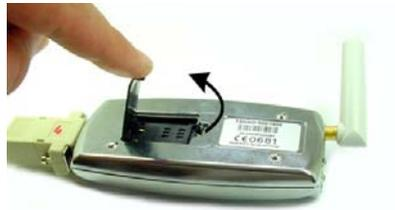
**Figure 9:** Open the cover cap.
