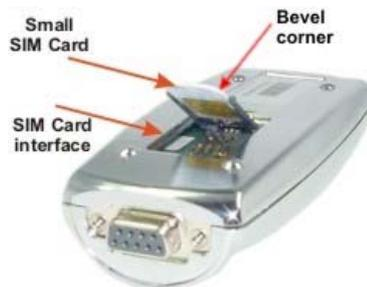
**Figure 6:** SIM interface (interface E)
