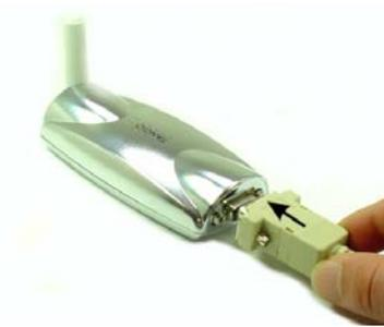
**Figure 12.b:** Connect 9pin serial to modem.
