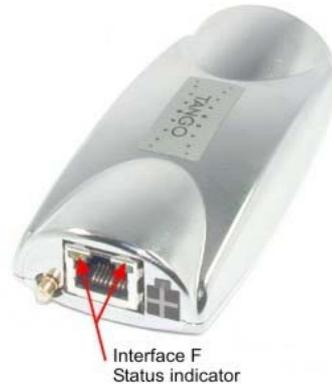
Figure 7: Status indicator of modem
