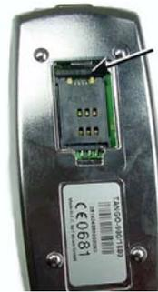
**Figure 10:** Push the inscription "PUSH ▲ OPEN" to open the SIM card holder.
