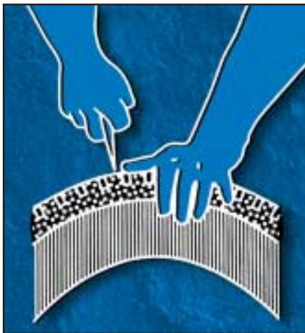
Figure 10.3 Dismount tire. Remove puncturing object. Using a probing awl, determine the size and extent of injury, and angle of penetration. Thoroughly inspect the inside of the tire for additional damage. Clean area to be repaired inside of tire with scraper and pre-buff cleaner.
