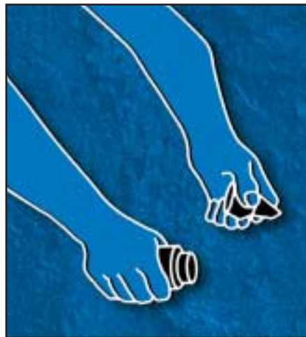
Figure 10.5 Apply a coating of chemical cure cement to the leading 1/3 of the cured plug. Remove the end of the plug insertion tool and insert the plug into the nose piece. Do not contaminate the plug or cross thread the nose piece.
