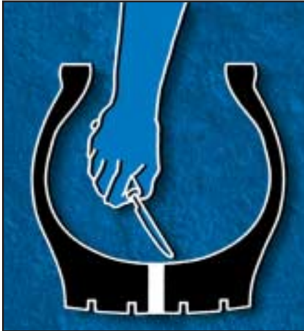
Figure 10.8 Cut excess plug 1/16" above the liner surface on the inside. Do not stretch plug.
