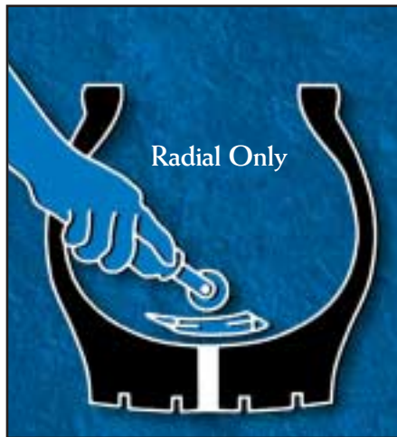
Figure 10.11 Place beads in a relaxed position. Center the patch over the plug and stitch the patch from the center out. Directional arrows on the patch must be properly aligned, after stitching is complete. Apply a coat of butyl liner repair sealer to the patch edges and the over buffed liner. Trim the excess plug no more than 1/8" above the outside tread surface.
