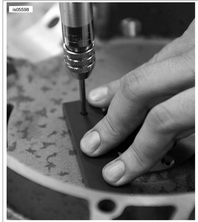
Figure 10. Tapping Lock Screw Holes
