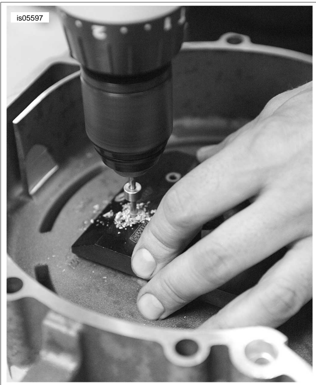
Figure 9. Drilling Mounting Screw Holes
