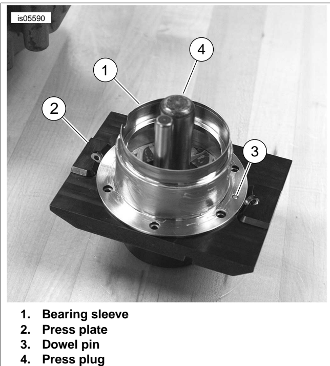
Figure 3. Bearing Insert and Press Plate
