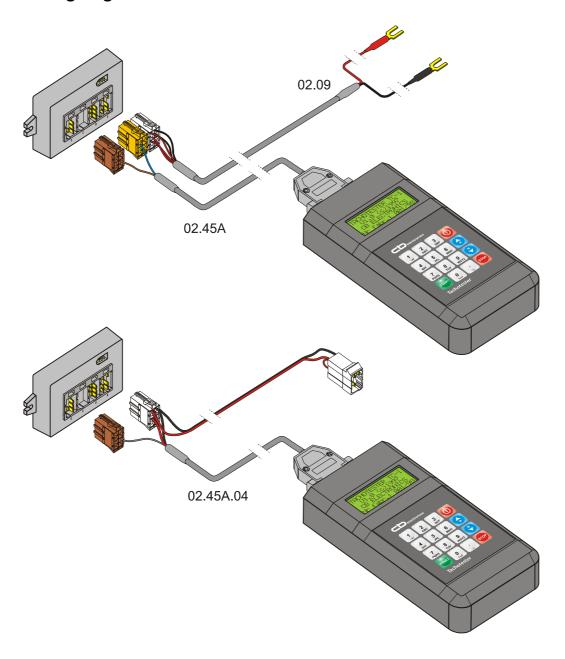
The simulator device is programmed using **TC-1 Tachotester** produced by CB Electronics. Connect the simulator to Tachotester using **02.45A** or **02.45A.04** cable. The simulator powered from external power supply, for example using **02.09** cable
