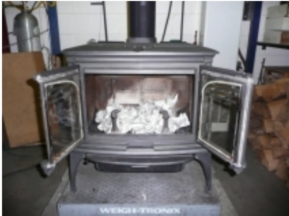
Crumple 6 to 8 full pieces of newspaper and place them in the center of the firebox.
