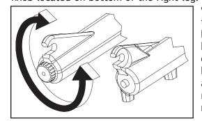
whereas, rotating the knob counter clockwise will reduce the damping. Excessive rebound damping will give you a harsh ride over repetitive bumps (like braking bumps) because the fork will pack up. Insufficient rebound damping will make the fork over active, top out and slap back when landing from a jump. We suggest that you try adjusting your fork on the very active side, minimum rebound. Then try it over a variety of terrain and tune in more rebound from there.
