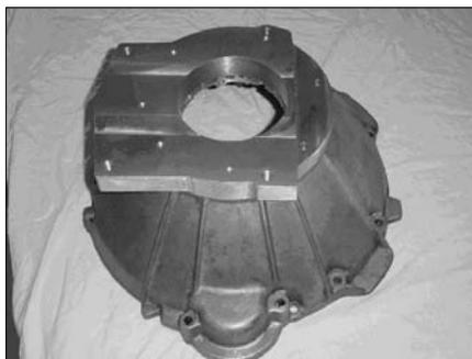
Figure 8 - Completed bellhousing
