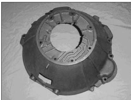
Figure 6 - Bored out auto bellhousing
