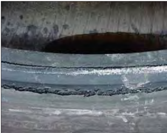
2nd stage - bead splitting from heat
