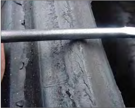
1st stage - turning of the bead
