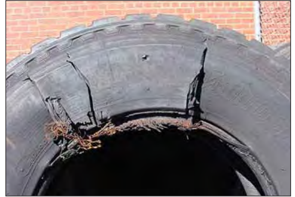
3rd stage - partial unwrapping of the casing ply
