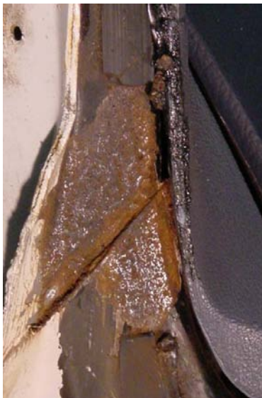
(Level 2 – 3 corrosion of pinchweld)
