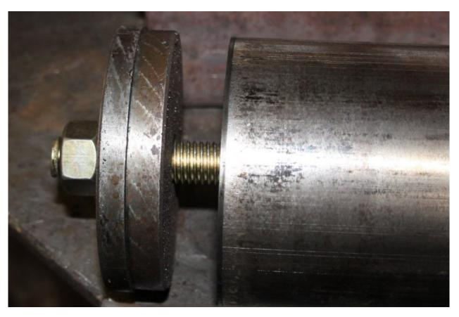
The puller must use an exact sized bottom plate. It must be stepped so that the top of the plate fits inside the liner with no play. The lower section must be slightly smaller then the OD of the liner. The step must be machined precisely to give an even pull.
