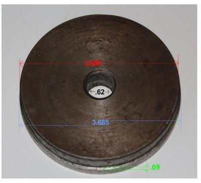
The following measurements are what we used but should be confirmed the best was to make a puller bottom, or have it made at a machine shop, is by using the actual of the new liners for measurements. The most important measurement is the outside OD - it must be as close as possible to the block bore size - it should be a tight fit.
