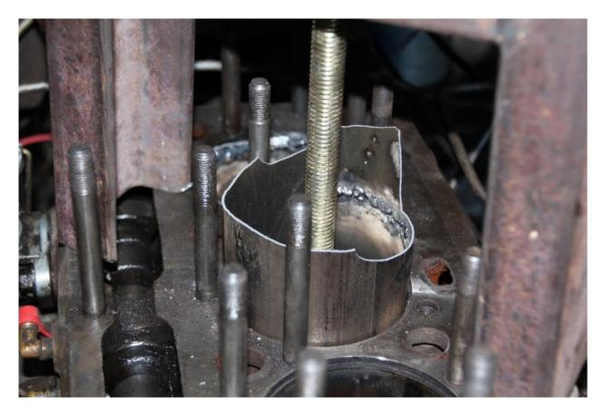
When the liner contacts the puller frame it should be broken off (they break very easily with a tap of a hammer) so that you can continue pulling. A tall pulling frame could be used but the taller it is the stronger it has to be and the longer the reddi rod. I found that a shorter puller and two pulling stages works best.
