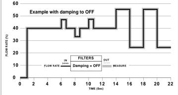
Damping function(OFF) extent follows the trend of fast flow
