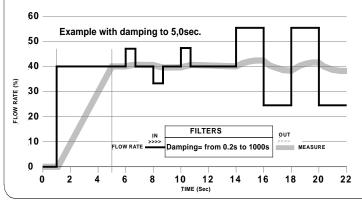
Damping mode based on time (from 0.2s to 1000s) The measure is averange over a number of samples determined by the value assigned to the function. When the damping parameter is expressed in seconds, the filter works damping the measurement noise and sudden change of flow rate. Increasing the parameter of damping increase the stability of the measurement.
