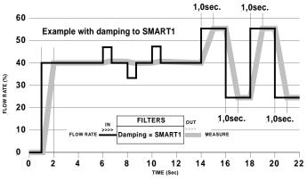
Damping(Smart 1,2,4):this does something effective filter measure noise and the sudden change in flow rate is measured by how smart damping parameter on the rise.
