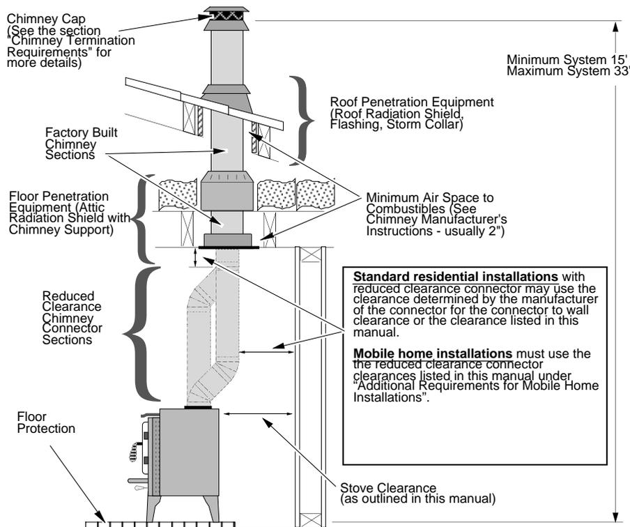
**Drafting Performance** This appliance relies upon natural draft to operate. External forces, such as wind, barometric pressure, topography, or factors of the home (negative pressure from exhaust fans, chimneys, air infiltration, etc.), may adversely affect draft. Travis Industries can not be responsible for external forces leading to less than optimal performance.
