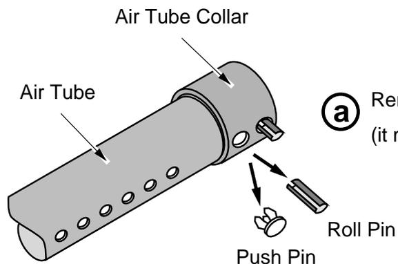
**a** Remove the left pin on the air tube collar (it may be a roll pin or push pin).
