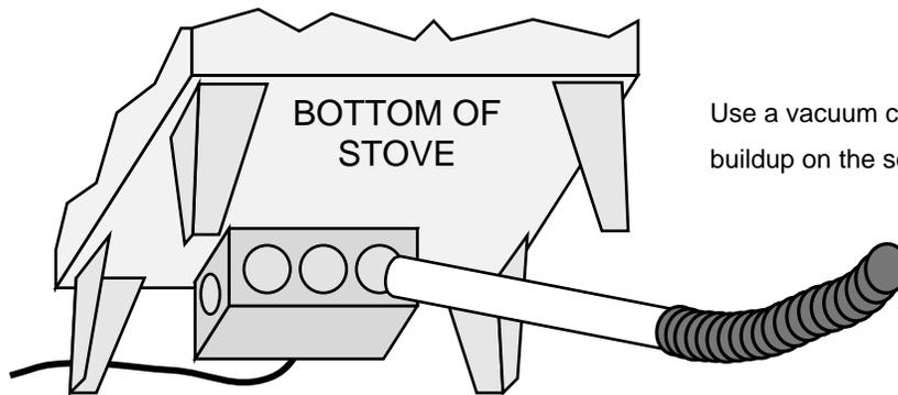
Use a vacuum cleaner to remove any buildup on the screens of the blower.
