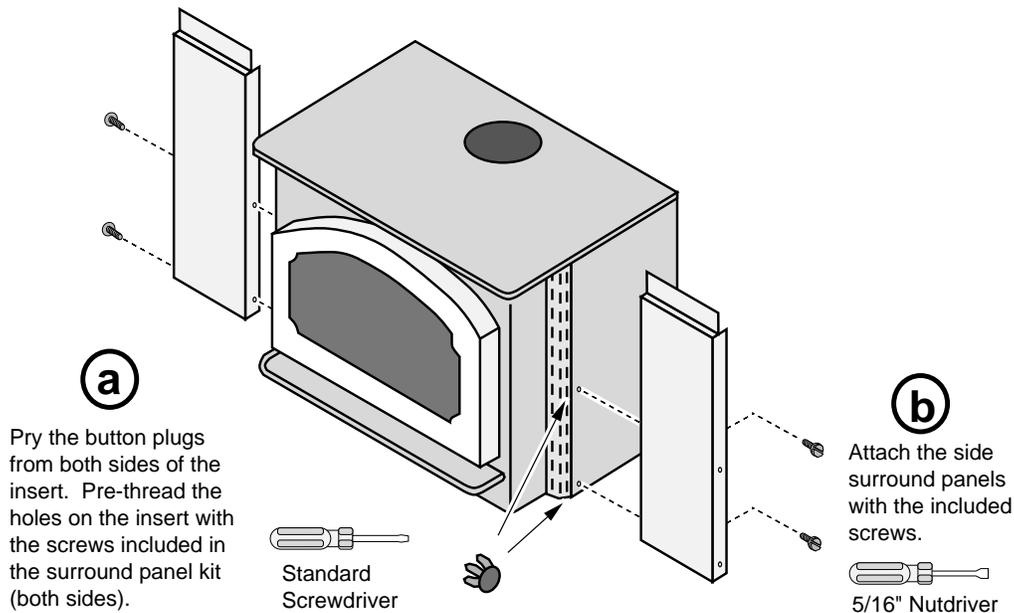
2. Adjust the position of the side panels so they are: 1) aligned with the top of the insert; 2) both the same distance back from the front of the insert; 3) perpendicular to the floor (use the top panel, if necessary, to judge alignment). Tighten the screws that hold the side panels in place.
