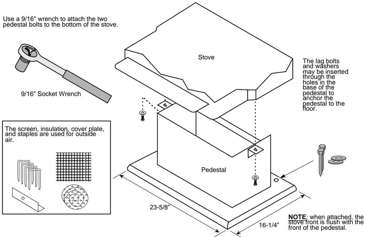
The screen, insulation, cover plate, and staples are used for outside air.
