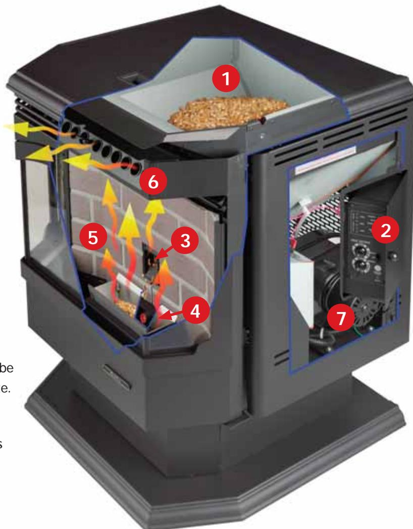
5. High pressure air is pulled into the base of firepot from the quiet combustion fan and forced through burning pellets. The variable speed control automatically allows the fan to be turned down in conjunction with the feed rate.
