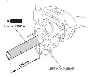
16. Spray isopropyl alcohol over the inside of the grip heater and outside of the left handlebar.
