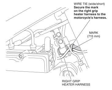
53. Secure the right grip heater harness using a wire tie as shown.
