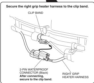
43. Remove the wire tie and dummy connector. <Right side>
