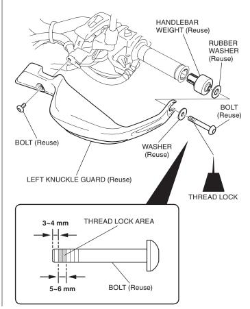
56. Check the throttle cables not to interfere with the knuckle guard as shown.
