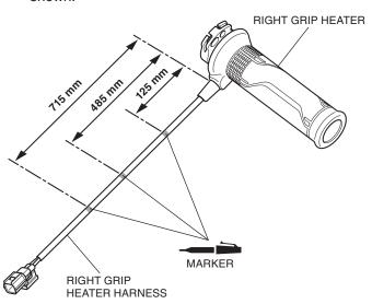
30. Wind the electrical tape on the marked position as shown.
