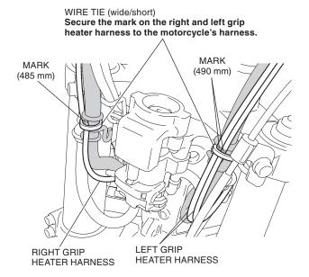
46. Secure the left grip heater harness using a wire tie as shown.
