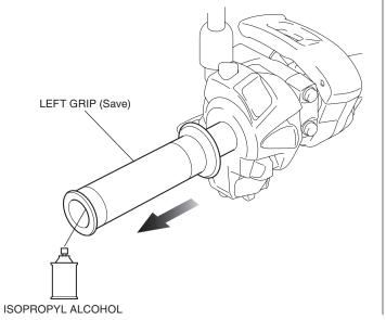
13. Using a isopropyl alcohol, remove all traces of adhesive from the left handlebar pipe.
