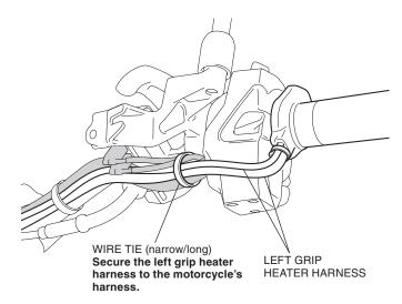
48. Secure the left grip heater harness using a wire tie as shown.
