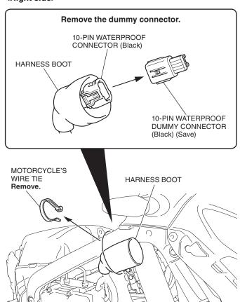
44. Connect the heater controller as shown.
