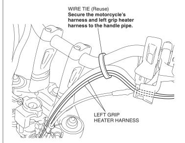
47. Secure the left grip heater harness using a wire tie as shown.
