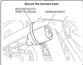
45. Secure the right and left grip heater harness using the wire ties as shown.
