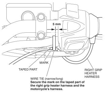
51. Secure the right grip heater harness using a wire tie as shown.
