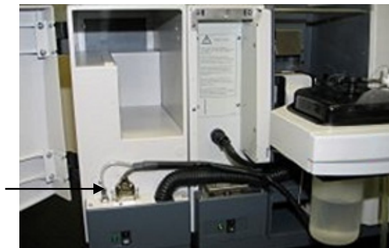
Figure 7 Location of the PSD gas and control cable connectors on the GTA
