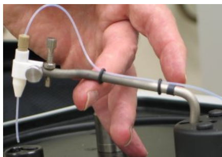
Figure 12 Capillary tubing in place
