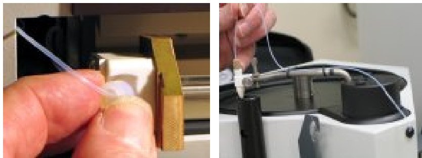
Figure 11 Connecting capillary at the block and threaded through the o-rings
