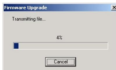
To ensure that the Vectrino firmware is not corrupted if the download transmission fails during the download process, the Vectrino runs a check on the received file before it is allowed to replace the existing firmware.
