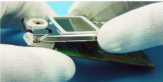
Separate the UI MODULE from the radio module.
