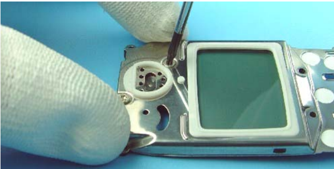
If it is needed to change the SPEAKER, release the TORX PLUS® screws size 6 as shown in the picture. When assembling use a torque of 8Ncm.
