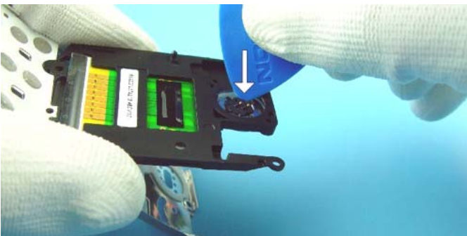
The SPEAKER can be changed separately. To remove it from the LCD Housing, push it with SRT-6. Do not damage the spring contacts.
