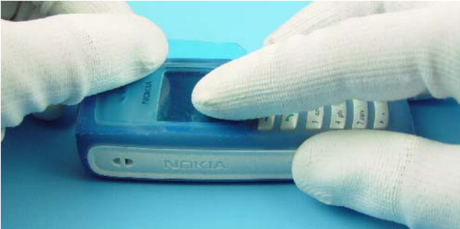
Protect the window with protection foil to avoid dust and scratches.
