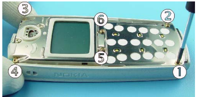
Unscrew the six TORX PLUS® screws size 6, using the order shown. For assembly, the reverse order and a torque of 17Ncm has to be used.
