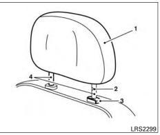
Non-adjustable head restraint/ headrest components
