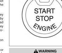
Do not operate the push-button ignition switch while driving the vehicle except in an emergency. (The engine will stop when the ignition switch is pushed 3 consecutive times in auick succession or the janition switch is pushed and held for more than 2 seconds.) If the engine stops while the vehicle is being driven, this could lead to a crash and serious injury.
