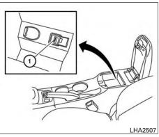
USB INTERFACE (models without Navigation System) (if so equipped)
