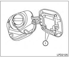
To remove the fuel-filler cap:
