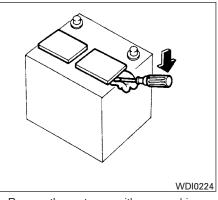
1. Remove the vent caps with a screwdriver as shown. Use a cloth to protect the battery case.
