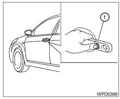
All doors will be locked automatically unless one of the following operations is performed within 1 minute after pushing the request switch.
