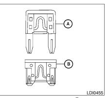
Two types of fuses are used. Type (A) is used in the fuse boxes in the engine compartment. Type (B) is used in the passenger compartment fuse box.
