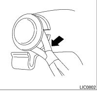
To install the cargo net, attach the net to the retainers.
