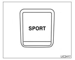
Adjusts the throttle sensitivity and transmission points (CVT only) to enhance performance. Press the SPORT button on the instrument panel to activate. The SPORT mode indicator light (on the speedometer) will illuminate. The SPORT mode indicator light will remain lit while the mode is active.
