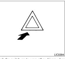
Push the switch on to warn other drivers when you must stop or park under emergency conditions. All turn signal lights flash.
