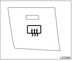
To defrost the rear window glass and outside mirror (if so equipped), start the engine and push the rear window defroster switch on. The rear window defroster indicator light on the switch comes on. Push the switch again to turn the defroster off.
