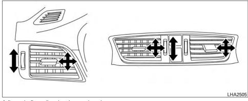
Adjust air flow direction by moving the vent slides.
