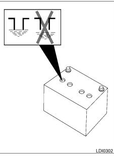
2. Check the fluid level in each cell. If it is necessary to add fluid, add only distilled water to bring the level up to the bottom of the filler opening. **Do not overfill.** Reinstall the vent caps.
