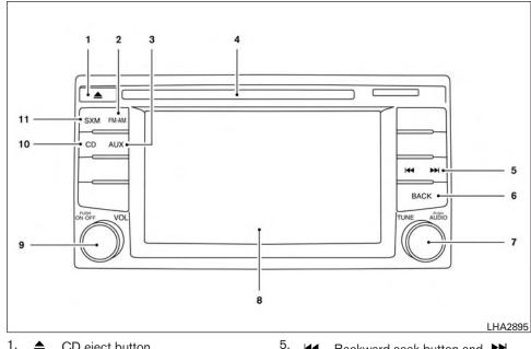
9. ON-OFF button / VOL (volume) control knob 10.CD button 11.SXM button\*
