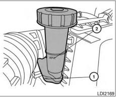
Check the fluid level in the reservoir. If the level is below the MIN line ①, or the brake warning light comes on, add Genuine NISSAN Brake Fluid or equivalent **DOT 3** fluid up to the MAX line ②. If fluid must be added frequently, the system should be checked by a NISSAN dealer.
