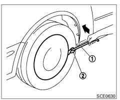
Removing the wheel cover (if so equipped)
