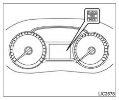
long as the low tire pressure warning light remains illuminated. For more information see "Low tire pressure warning light" in the "Instruments and controls" section, "Tire Pressure Monitoring System (TPMS)" in the "Starting and driving" and "Wheels and tires" section in the "Maintenance and do-it-yourself" section of this Owner's Manual.
