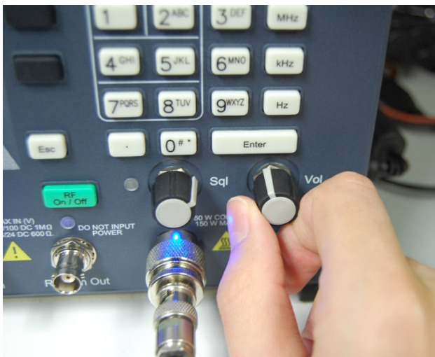
Figure 4-2. Adjust analyzer volume until about 4 kHz deviation is measured.
