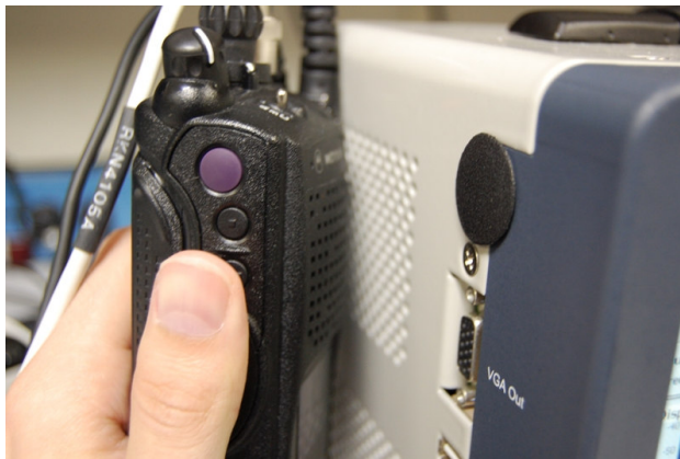
Figure 6-1. Place keyed radio next to analyzer speaker.
