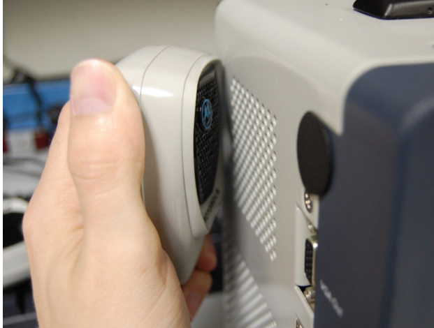
Figure 4-1. Place keyed microphone next to analyzer speaker.
