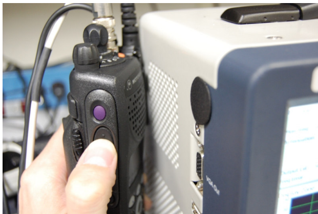
Figure 8-1. Place keyed radio next to analyzer speaker.
