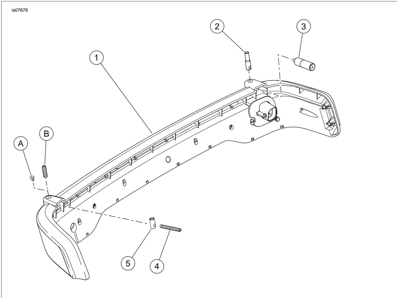
**Figure 2. Service Parts, Tour-Pak Smoked Wrap-Around Light Kit**
