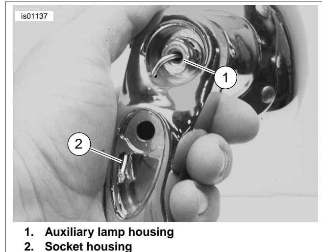
Figure 3. Auxiliary Lamp Wire Routing
