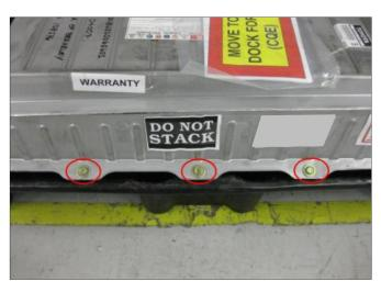
5. Securely fasten the HV Battery metal cover to the base of the battery with **all original** fasteners.
