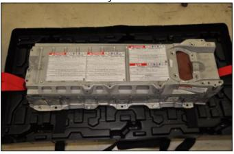
1. Place the battery in the center of the DRC.
