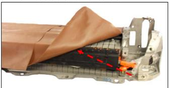
3. Using the HV insulation Mats supplied with the DRC, completely cover the bus bar covers.
