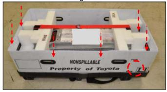
5. Install the corrugated sleeve onto the base pallet. Press down firmly to ensure proper fit.
