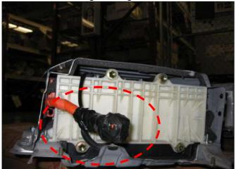
2. Cover all exposed high voltage cables, wire harnesses and or terminals with UL-listed non-conductive black electrical tape.
