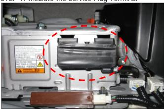
Cover the hybrid battery service plug terminal with UL-listed non-conductive black electrical tape.
