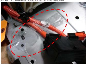
4. Using packaging tape, secure all hybrid cables and wiring harnesses to the battery base plate.
