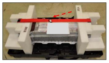
4. Tighten the red strap securing the foam in the DRC.
