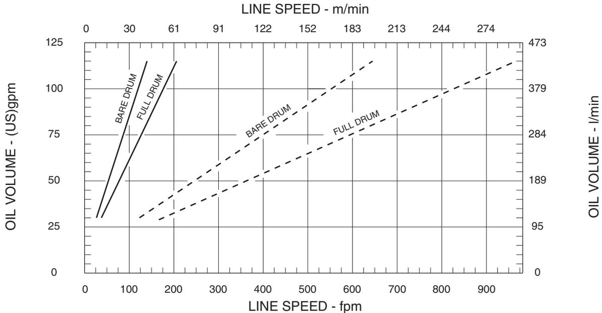
Performance graphs are based on standard hydraulic motor, gear ratio and cable drum with 7/8 inch diameter wire rope.
