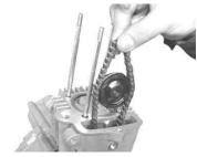
Install the cam chain guide roller with a sealing washer, and tighten the guide roller bolt temporarily.
