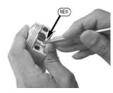
Attach the piston pin circlip so the ring end gap does not meet with the notch on the piston pin hole, and it should be either on the top or at the bottom of the hole as illustrated in the figure below.
