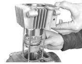
Compressing the piston rings, install the cylider with care not to get the ring-end gaps out of alignment.
