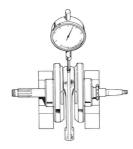
• Measure the misalignment on the journal bearing of the crank shaft.
