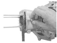
Loosely tighten an original hex bolt which holds the crankcase on the cylinder side.
