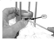
Attach the piston pin circlip so the ring end gap does not meet with the notch on the piston pin hole, and it should be either on the top or at the bottom of the hole as illustrated in the figure below.
