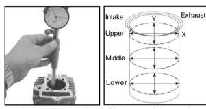
In case the cylinder wall is beyound the service limits, change the cylinder and piston at the same time as a set.
