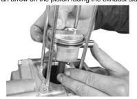
Plug the sleeve hole and the cam chain hole on the crankcase with a clean cloth, and fix a piston pin circlip.
