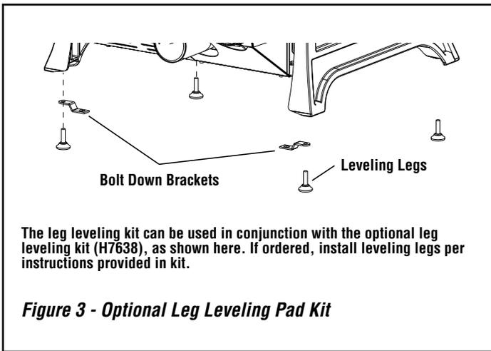
**Figure 3 - Optional Leg Leveling Pad Kit**
