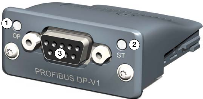
Figure 2-10. Profibus Status LED Module
