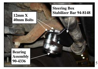
11. Tighten the hardware so it is snug. Torque the **10mm** sway bar mounting to 40 ft./lbs.
