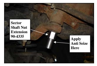
Insert the 12mm X 40mm bolts through the top of the steering box stabilizer bar (94-8184). Install the bearing assembly (90-4336) onto the sector shaft extension nut (90-4335) and 12mm bolts. Secure using the 12mm washers and nuts.
