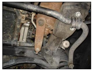
3. Carefully, unbolt the sway bar mounts from the frame. Be sure to support he sway bar so it doesn't swing down.
