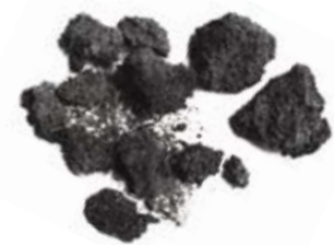
Above is an example of a pellet “clinker”. This mass of impurities can reduce airflow through the UltraGrate and create an unsafe burning condition.
