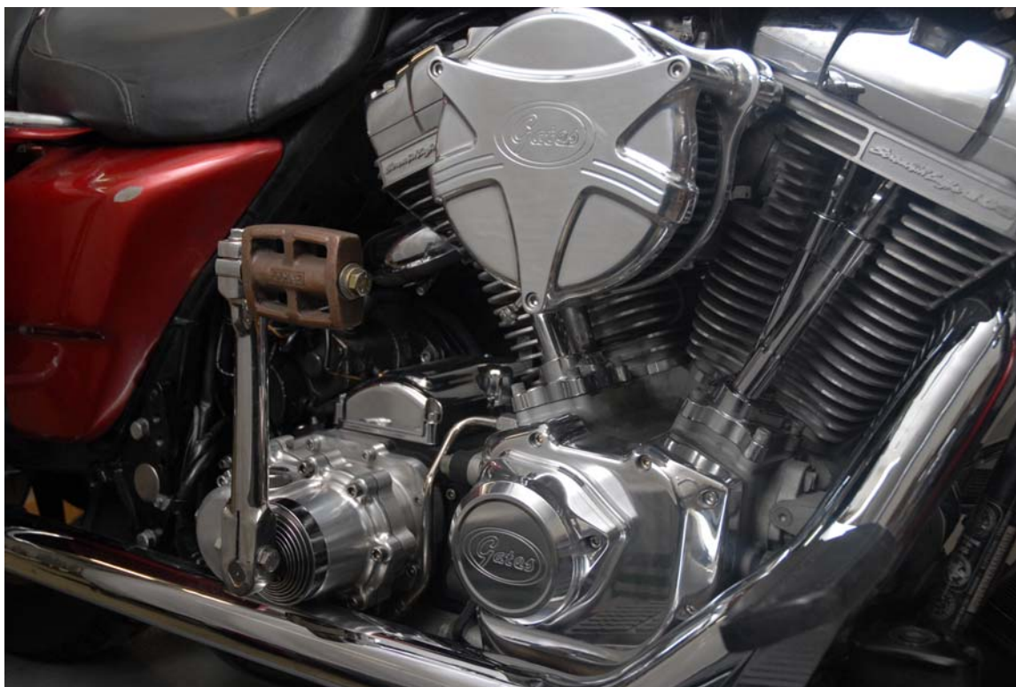
BAKER Drivetrain's 1999 Road King w/Part Numbers: FT106SL (Frankentranny Kit), 478-56CP-U84 (Kicker Cover), 3511-64 (Kick Arm/Pedal Assembly), 475-56P (Oil Spout Assembly), and 5011(Gates Ignition Kit)
