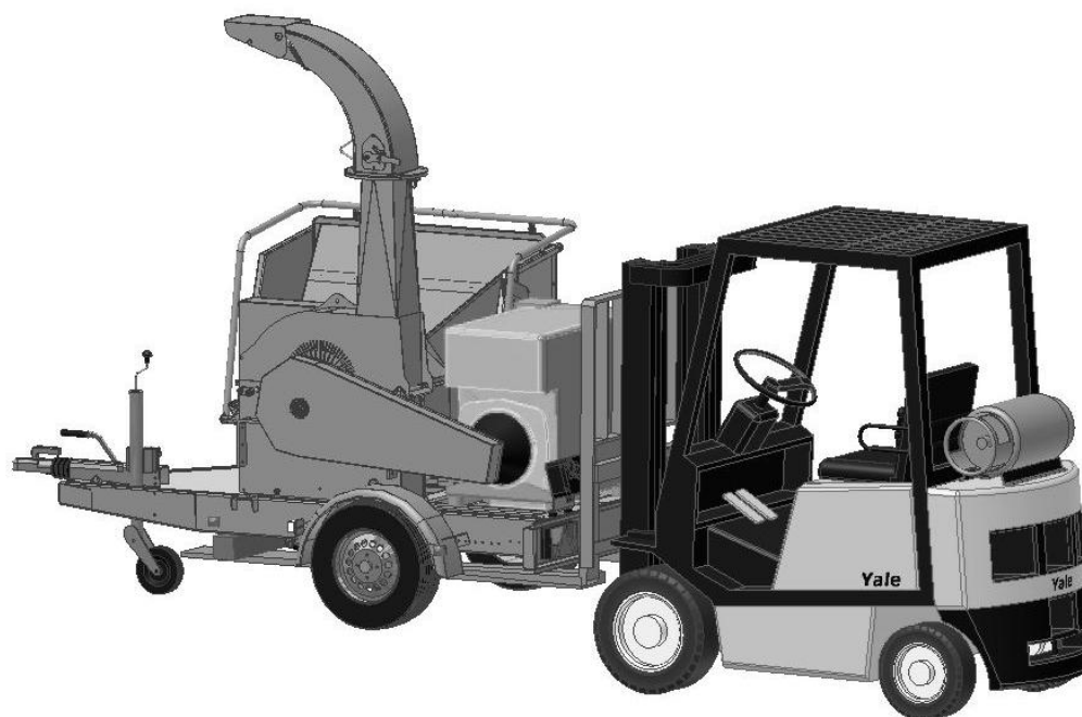
Figure 5 Lifting with a fork lift truck
