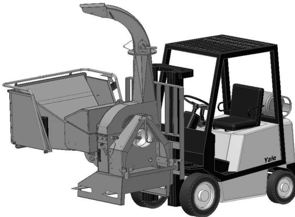
Figure 4 Lifting with a fork lift truck
