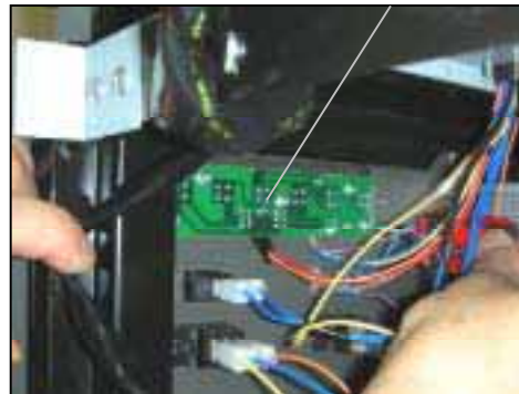
Display PCB Control PCB
