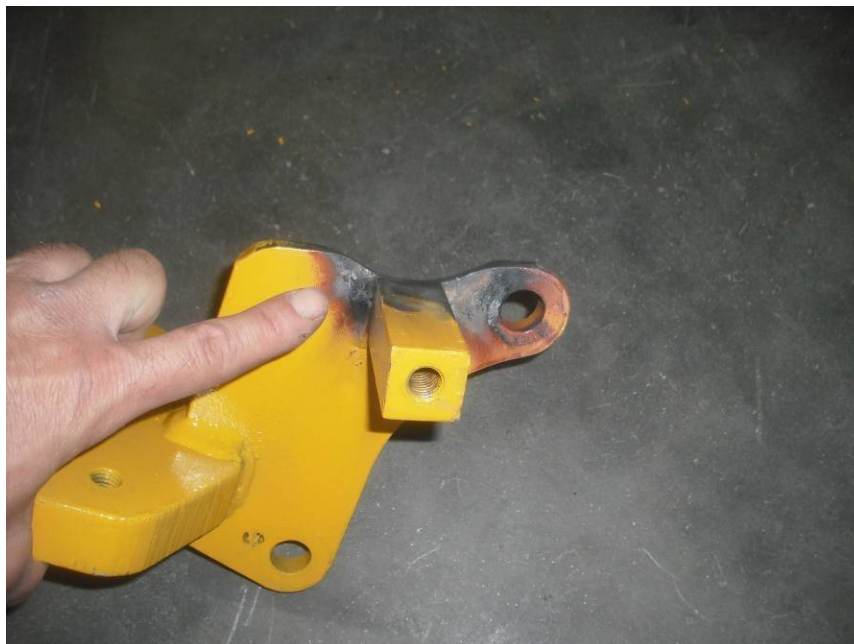
Figure 4: Motor Mount Modification
