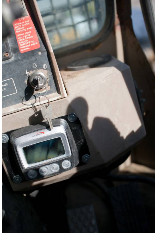
Figure 13: Modified Instrument Panel with PowerView
