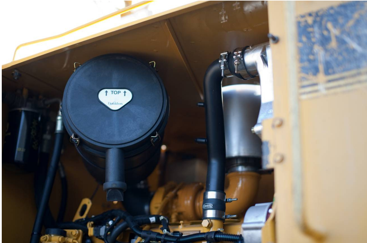
Figure 28: Cold CAC Tube Mounting
