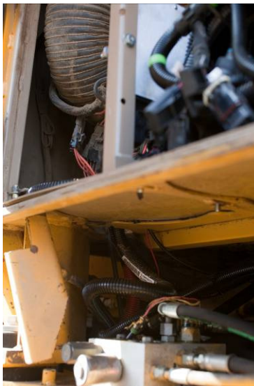
Figure 8: Rear Left Wiring Harness Routing
