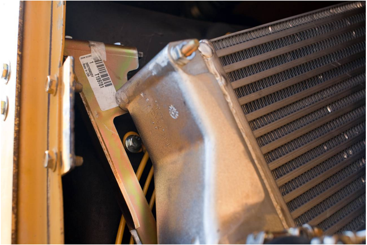
Figure 24: CAC Mounting to Left Side of Hood
