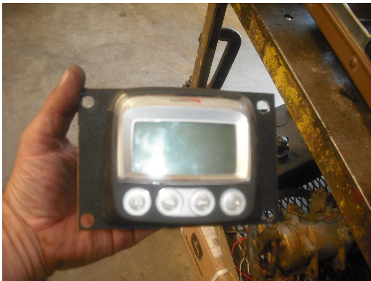
Figure 15: Power View Mounting Plate Front Side
