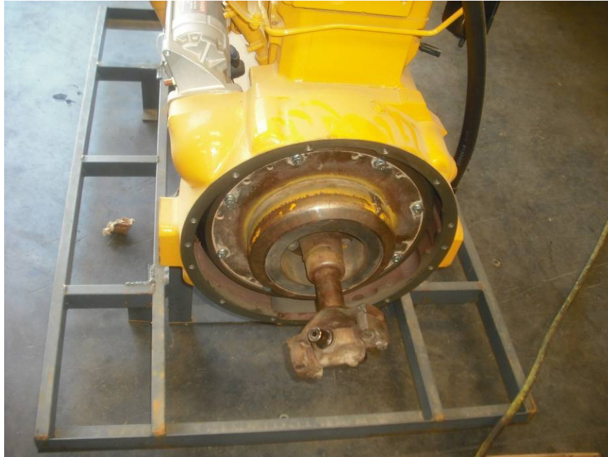
Figure 1: Installed Drive Adapter on New Engine
