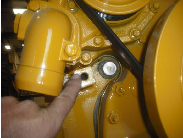
Figure 5: Front Right Motor Mount Installed on New Engine
