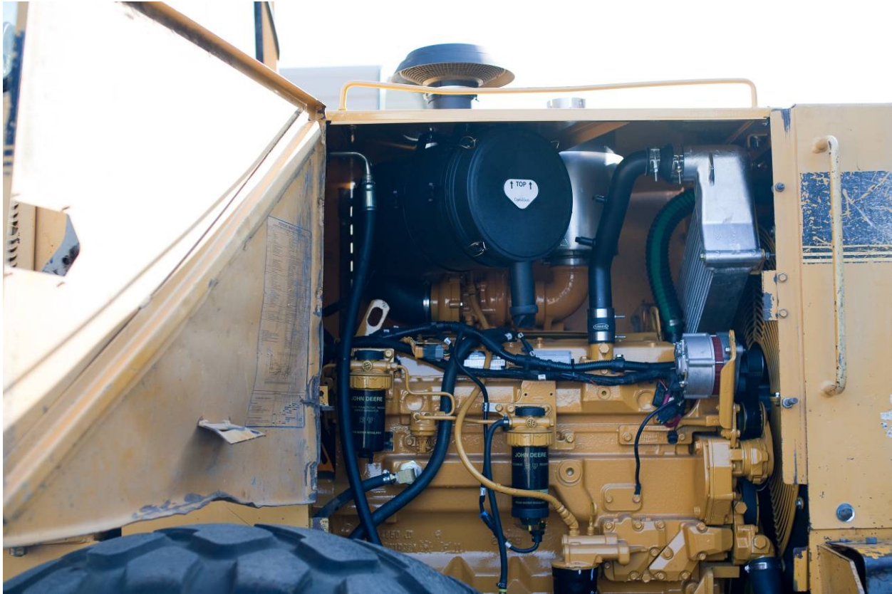
Figure 26: Air Cleaner Mounting To Underside of Hood
