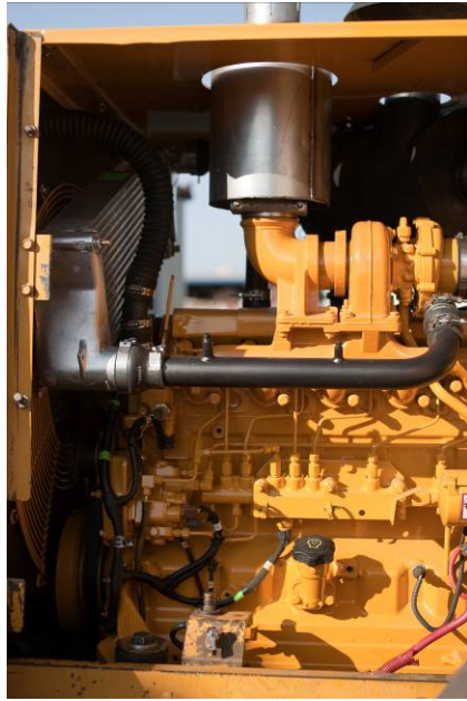
Figure 23: Muffler Mounting Location
