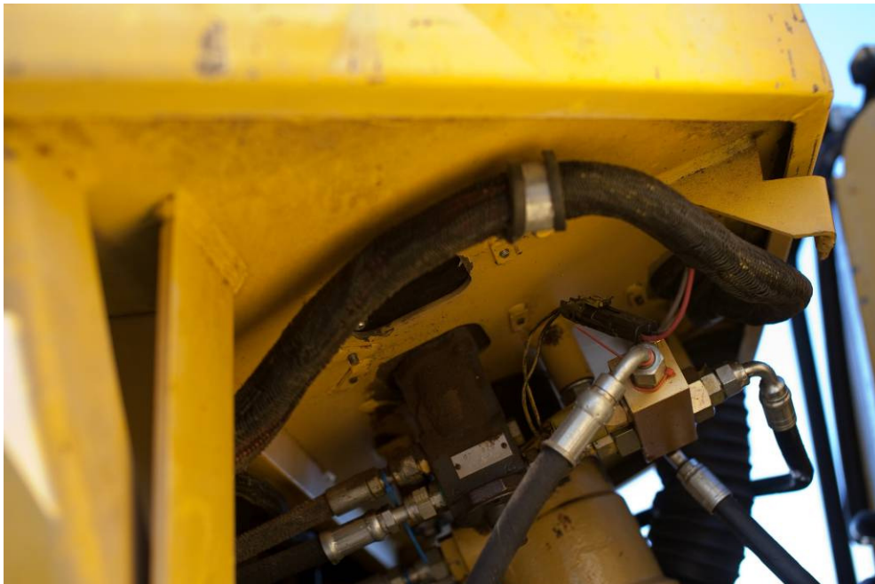
Figure 19: Underside of Accelerator with Potentiometer
