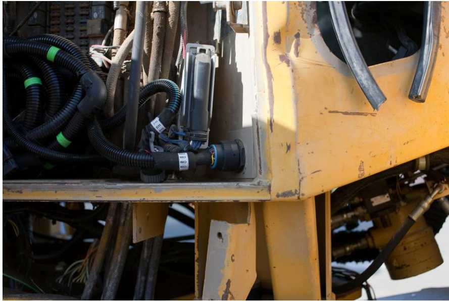
Figure 11: Harness Routing Through ECU Compartment
