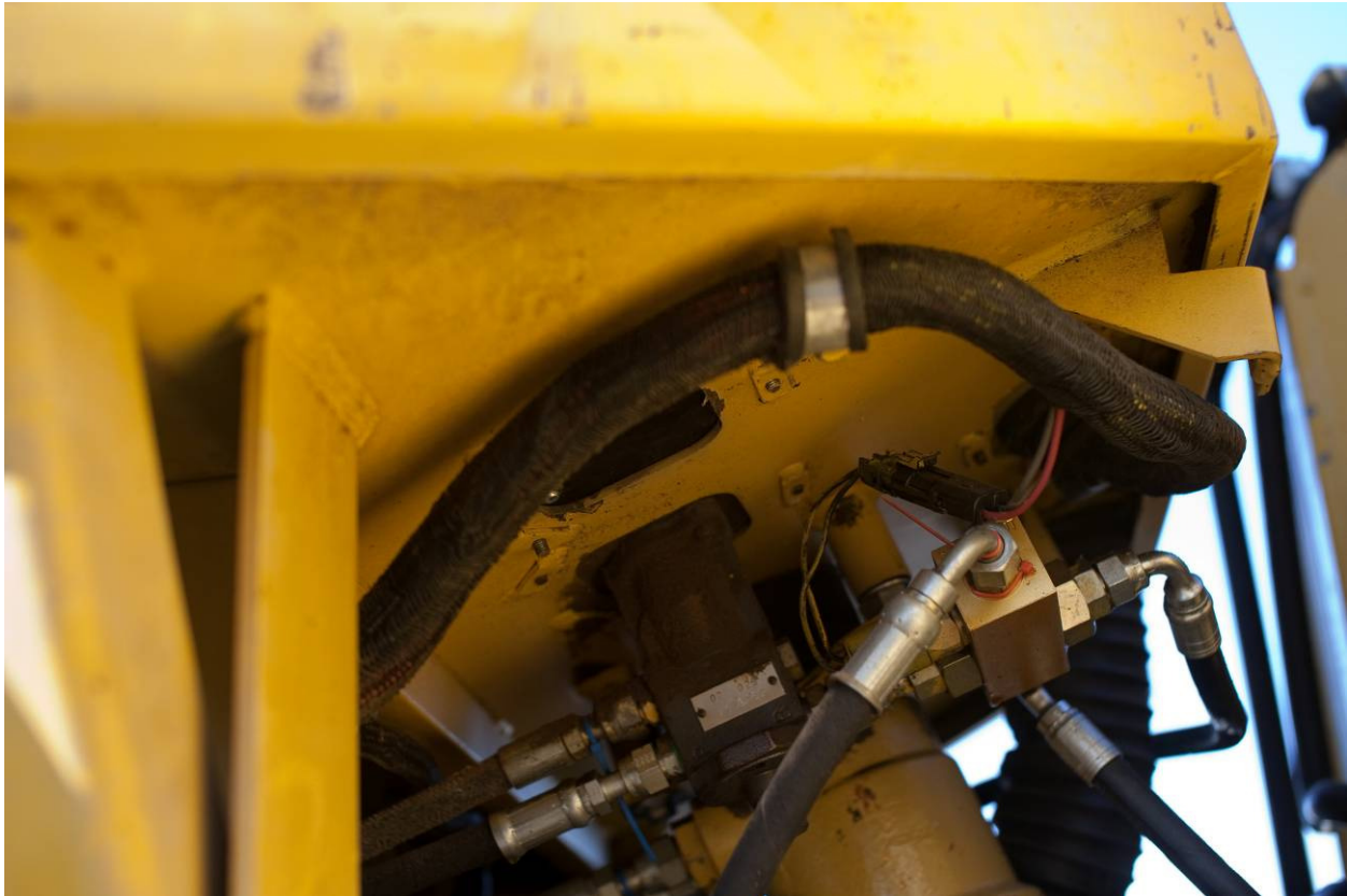
Figure 16: Wiring Harness Routing Under Cab
