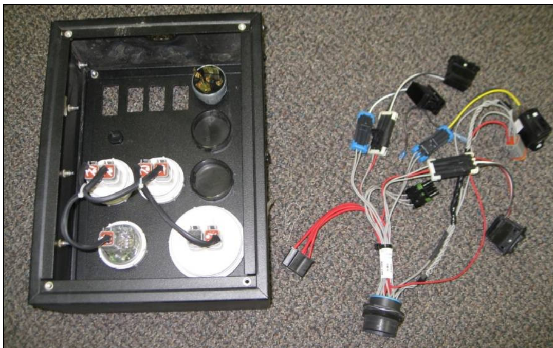
Figure 14: RE534022B Instrument Panel Harness
