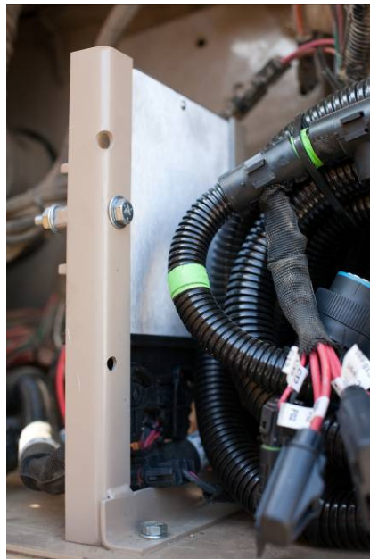
Figure 10: ECU Mounting Bracket
