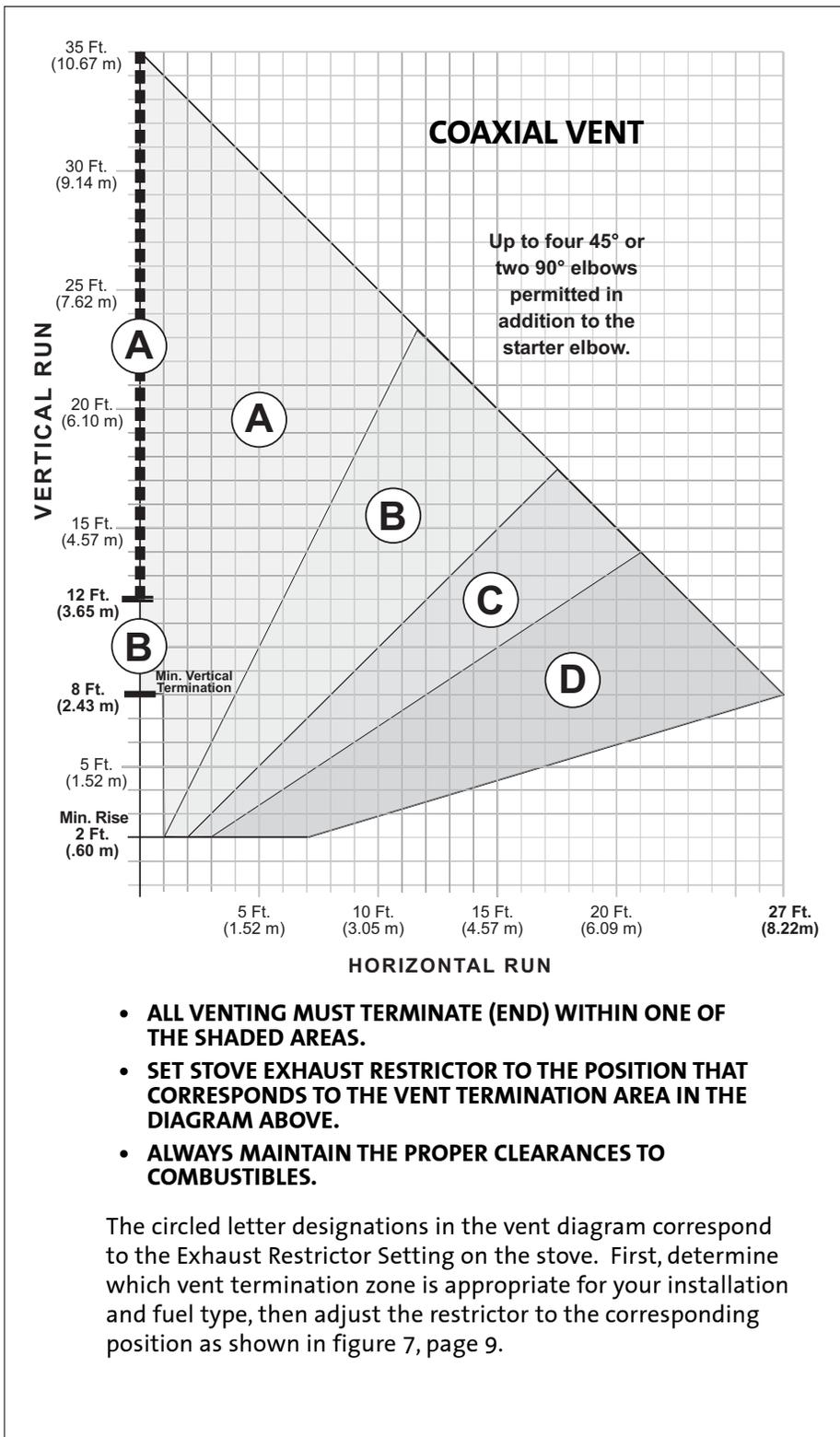
Figure 9. Coaxial Vent Termination Window / NG
