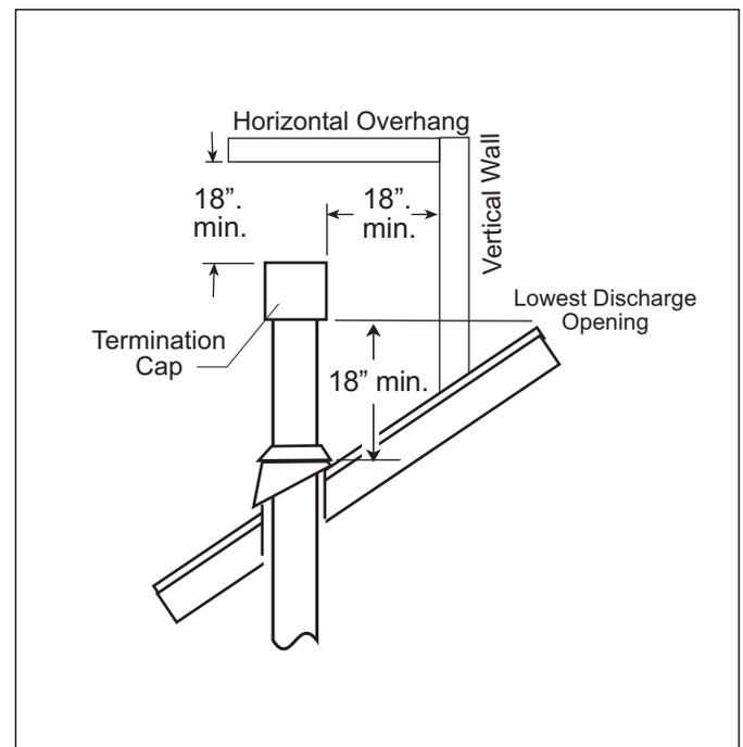
Figure 8. Vertical vent termination height above roof.
