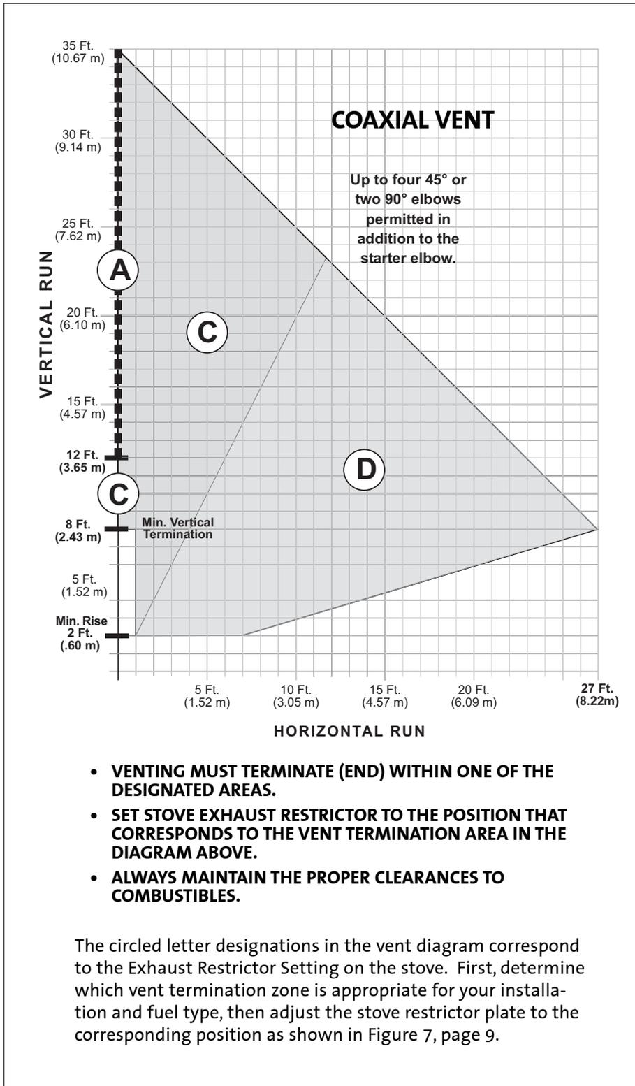
Figure 11. Coaxial Vent Termination Window / LP
