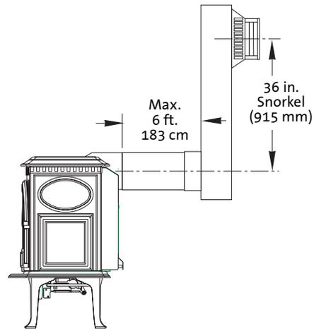
Figure 18. Maximum Horizontal with 36" Snorkel Termination.
