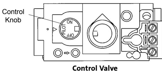
5. Push in gas control knob slightly and turn clockwise ➡ to "OFF".
