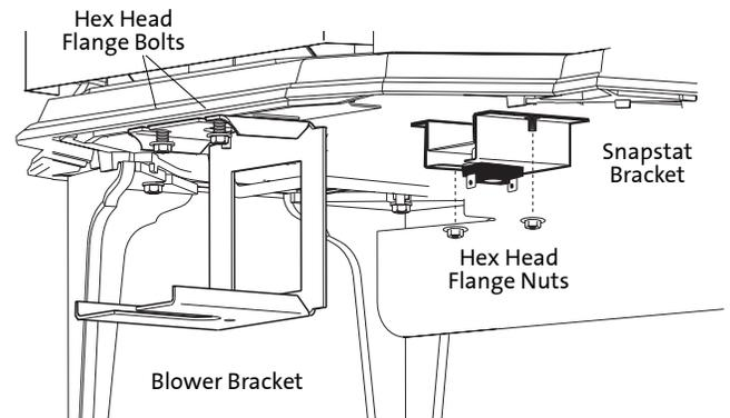
Figure 43 . Attach Snapstat and Blower Brackets.
