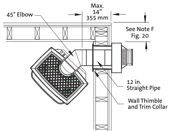
Figure 19. Corner Installation with 14" Snorkel Termination.
