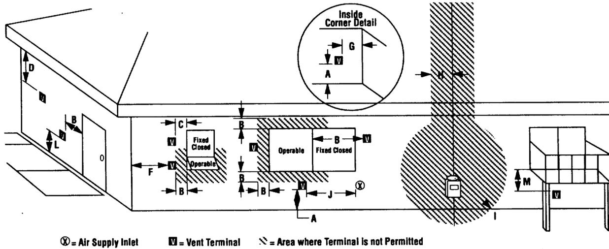
Figure 20. Vent Terminal Clearances - National Fuel Gas Code.
