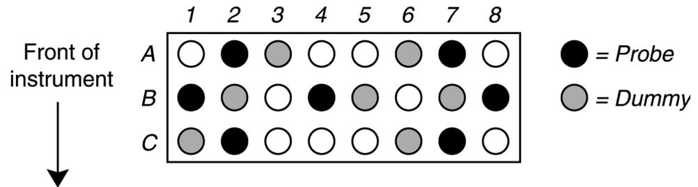
**Figure 2-6** Location of wells used in Temperature Non-Uniformity test
