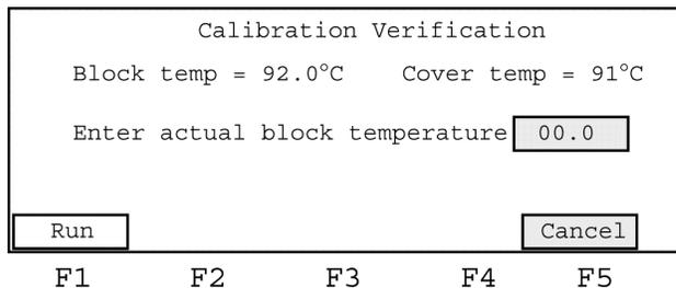
**Figure 2-3** Setpoint screen for entry of digital thermometer readings
