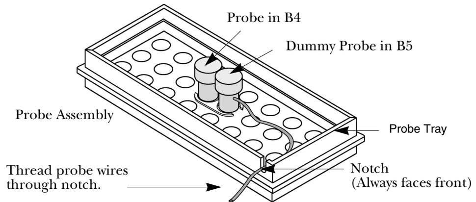
**Figure 2-1** RTD Probe Assembly
