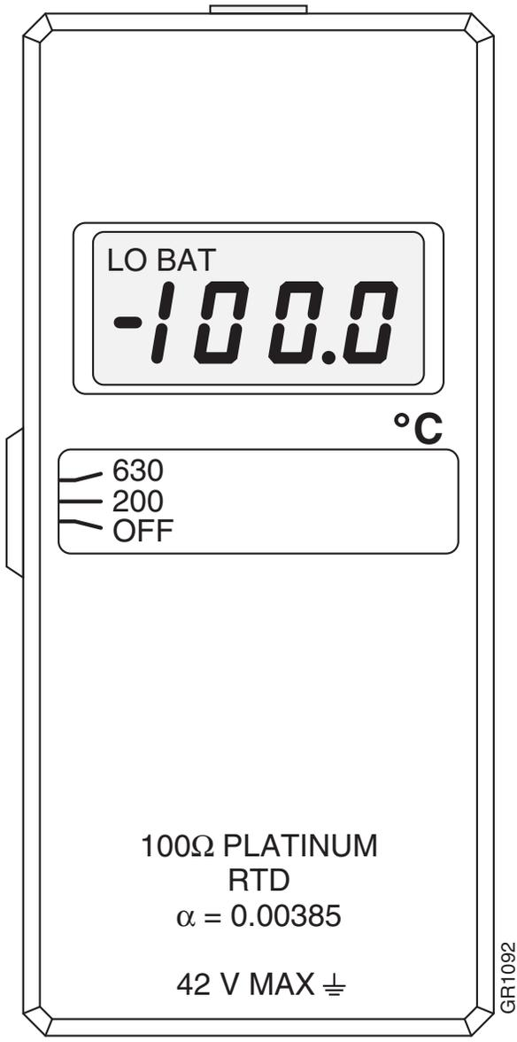
**Figure 1** Front view of digital thermometer
