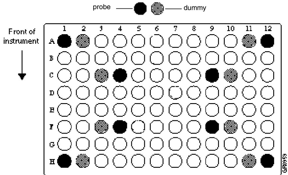
**Figure 4-1** 9700 Sample Block Wells for TNU Measurement
