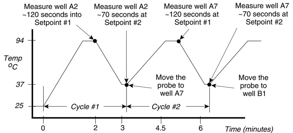
**Figure 2-4** The Temperature Non-Uniformity test
