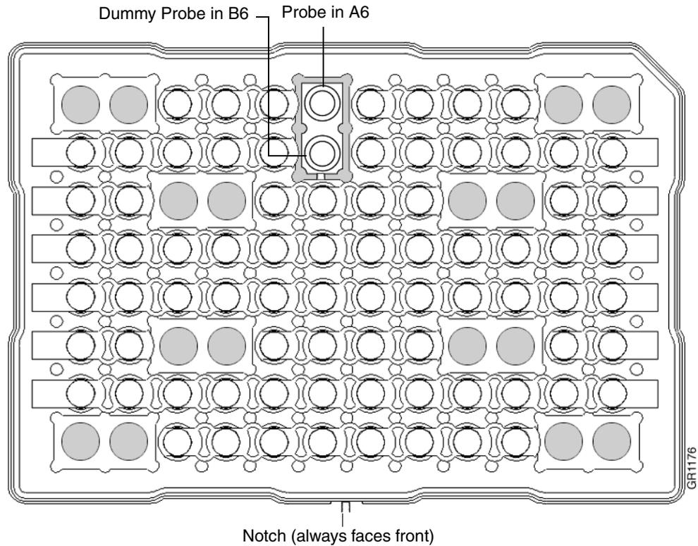
**The Tray Assembly** The 9700 temperature verification system is equipped with a tray assembly that ensures accurate measurement of temperature during the calibration verification and TNU procedures. The tray consists of a 96 well plate with caps. There are nine locations where no caps are present. One location is for the calibration verification test and the other eight locations are for TNU testing.
