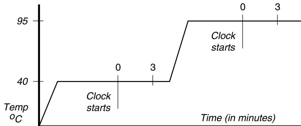
**Figure 3-1** Temperature measurements in the temperature calibration verification test
