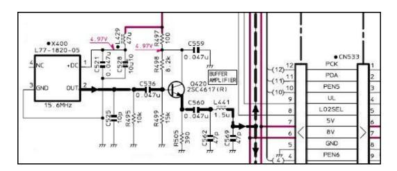
Figure 1 - Reference Oscillator Circuit Diagram
