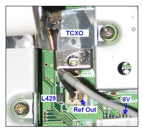
Figure 2 – Reference Oscillator Component Layout
