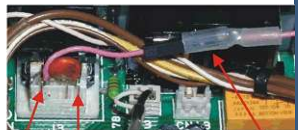
Pin2 GND Back side of ACC2 Connector AUX Key Line Conn Figure 4
