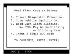
You have to count the MIL flashing on the dashboard and manually input the DTC number to MULTISCAN P2 to view the details as below:
