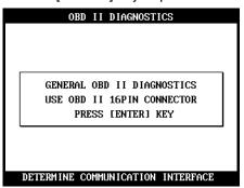
c MULTISCAN P2 then automatically tries to establish communication with the powertrain control module using standard OBD2 communication protocols in turn.
