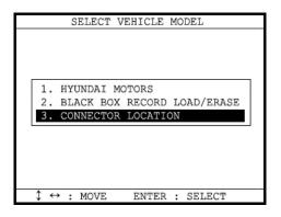
b Select [CONNECTOR LOCATION] from the vehicle selection menu if the adapter is not found in the place where it is supposed to be.
