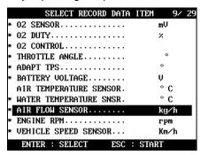
c You can select up to 40 PIDs to record. Press the [ESC] key when the selection is completed, then MULTISCAN P2 will start recording data.
