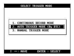
Before DTC, you will see the Live Data of the selected parameters keep refreshing, however, once triggered by DTC or [ESC] key stroke, only the percentile process information and sampling frequency will be displayed.
