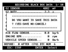
b When pressed [YES], a dialog box follows and asks you to input the test date. Enter the date and press the [ENTER] key to save the recorded data to MULTISCAN P2 memory.
