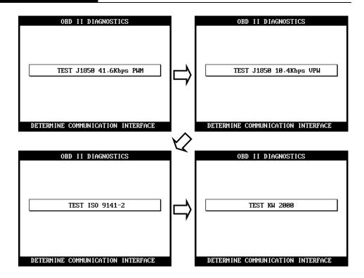
d When succeeded in communicating with the control module with any of these 4 standard protocols, MULTISCAN P2 reports the successful establishment of communication and waits for your command to commence generic OBD2 diagnosis as below:
