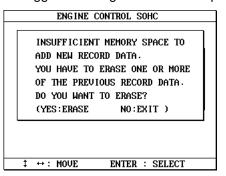
b. Press the [ERASE] key to proceed, then a list of saved data will follow. Locate the highlight bar on data to delete, and press the [ENTER] key. A query for your confirmation will follow. Press the [YES] key to erase otherwise press the [NO] key.
