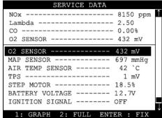
b. You can select up to 3 items in the same way and view the readings in graphic form by selecting [1. Graph] during the data stream display.
