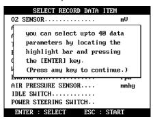
b MULTISCAN P2 will show you the whole live data parameters available in the control system you selected. Locate the highlight bar on the desired parameter and press the [ENTER] key.
