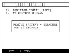
Removing the battery terminal will get rid of all information contained in the car stereo and other electronic devices. And it may not effectively erase the fault codes in some cars. Refer to the original repair manual for further information.
