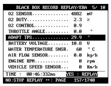
d. Pressing the [NO] key will stop replaying. You can restart replay by pressing the [YES] key again, but it will start from the first frame.
