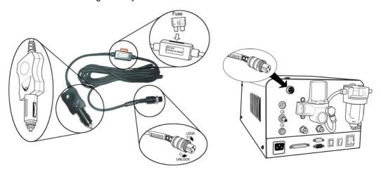
c Gas analyser begins to warm-up when power is supplied. Warming up takes 4 to 6 minutes in normal condition. It may take up to 15 minutes when it is cold and it is dependent to the actual air temperature.
