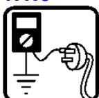
Megger test to check insulation.
