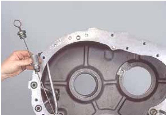
Figure 61 Dipstick and dipstick housing removed.
