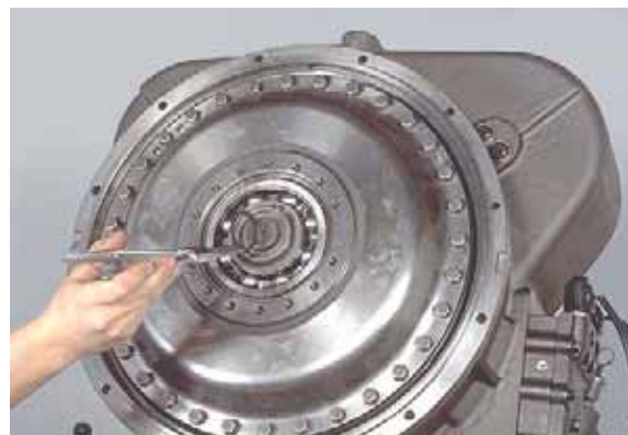
Figure 5 Remove turbine shaft outer retainer ring.
