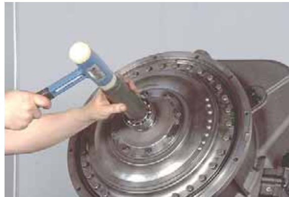
Figure 12 Tap input shaft bearing in place.
