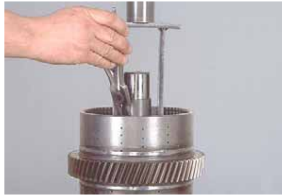
Figure 88 Compress piston return spring. Remove return spring retainer ring.
