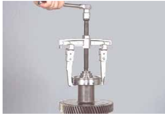
Figure 133 Remove clutch shaft rear bearing.
