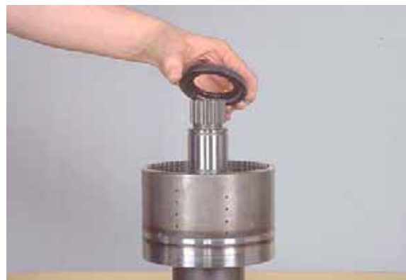
Figure 198 Remove spring retainer.
