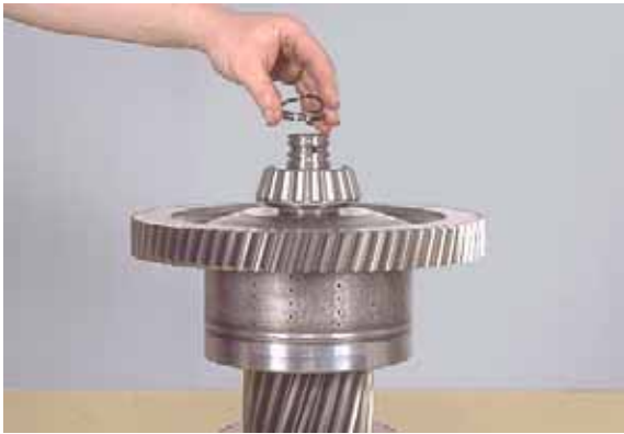
Figure 153 Remove clutch shaft oil sealing rings (piston rings).
