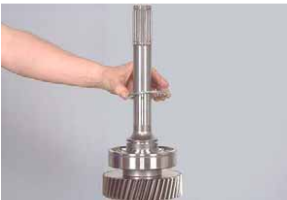
Figure 253 Remove front bearing washer.
