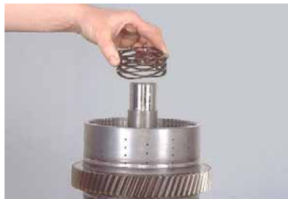
Figure 90 Remove piston return spring.
