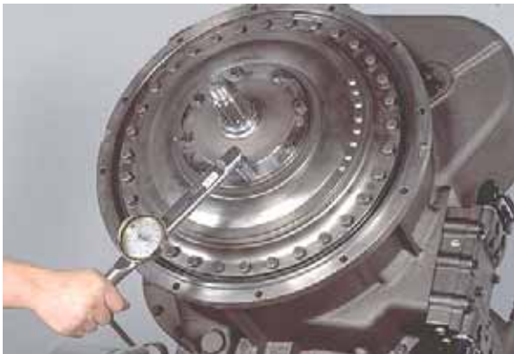
Figure 10 Install input shaft on impeller cover. Install input shaft bolts, tighten 37 - 41 ft. lbs. torque (50.2 - 55.5 N.m.).
