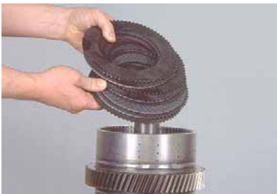
Figure 87 Remove inner and outer clutch discs.
