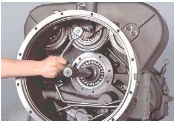
Figure 21 Remove pump drive gear bearing support bolts.
