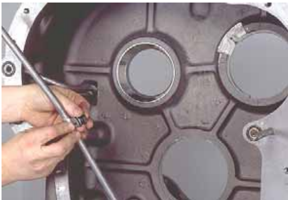
Figure 62 Dipstick tube, clip and screw removed.
