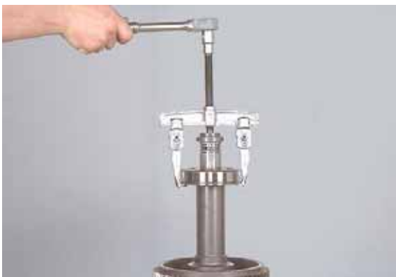
Figure 220 Remove 4th shaft front bearing.
