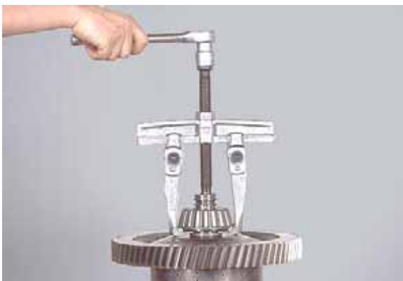
Figure 155 Remove rear bearing.
