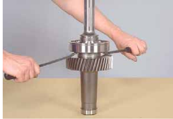
Figure 254 Pry front bearing from shaft.
