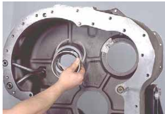
Figure 65 Remove low clutch shaft front bearing cup baffle plate and retaining.
