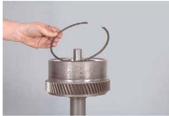
Figure 221 Remove end plate retainer ring.
