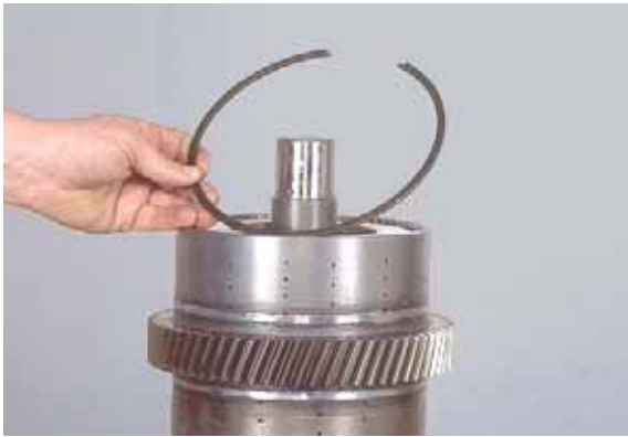
Figure 85 Remove end plate retaining ring.
