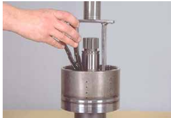
Figure 197 Compress piston return spring. Remove spring retaining ring.
