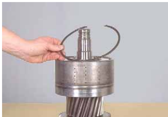
Figure 158 Remove end plate retaining ring.
