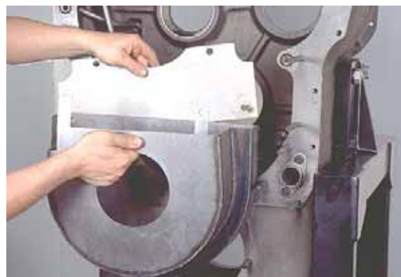
Figure 60 Oil baffle removed.
