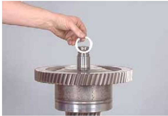
Figure 156 Remove gear thrust washer.
