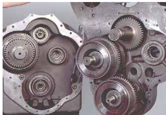
Figure 24 Separate converter housing from transmission assembly. Note: reverse and 2nd, and forward high and 4th clutch will remain in the converter housing.
