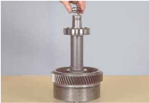
Figure 218 Remove clutch shaft oil sealing rings (piston rings).
