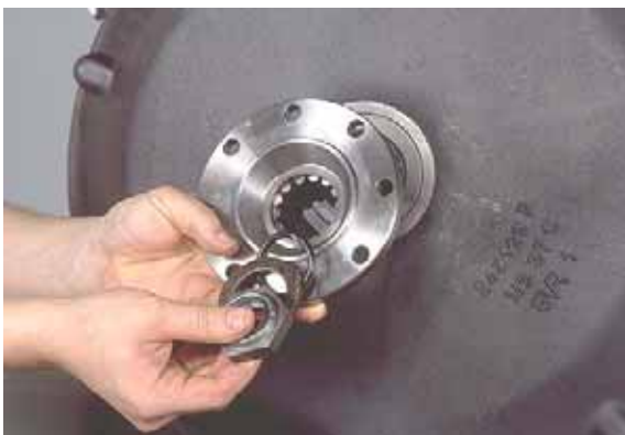
Figure 2 Remove input flange nut, washer and "O"-ring.
