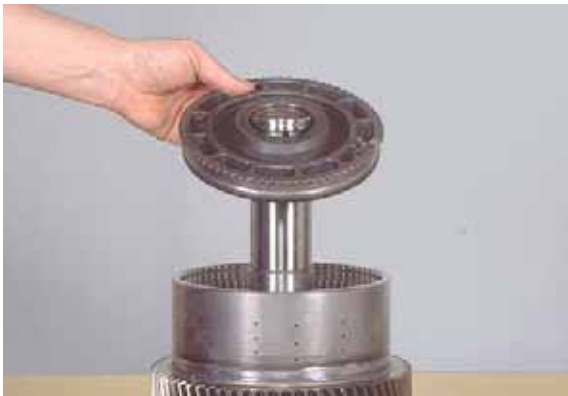
Figure 131 Remove clutch piston.
