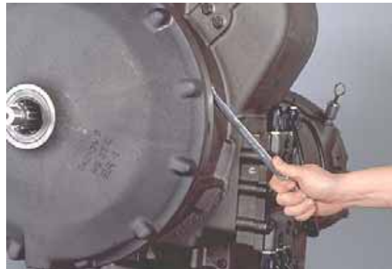
Figure 4 Remove bolts and lockwashers securing converter housing front cover to converter housing.
