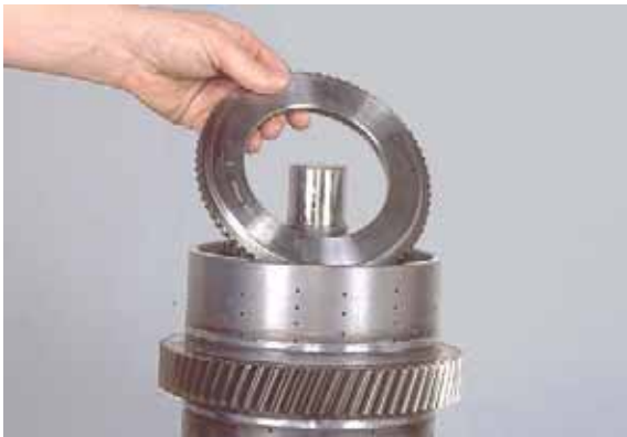
Figure 86 Remove end plate.
