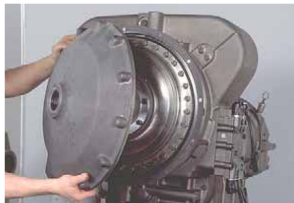
Figure 5 Remove converter housing front cover.
