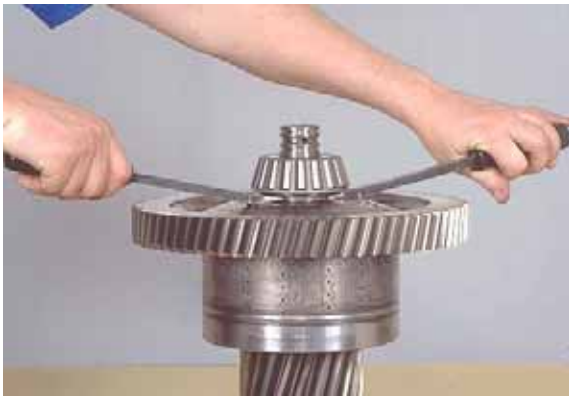
Figure 154 Pry rear taper bearing up, far enough to use a bearing puller.
