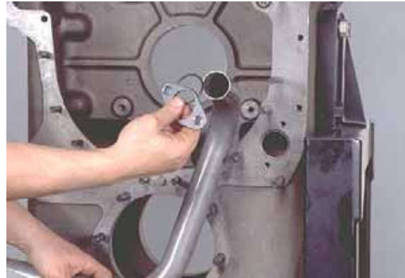
Figure 64 Suction tube, "O"-ring and retainer removed.
