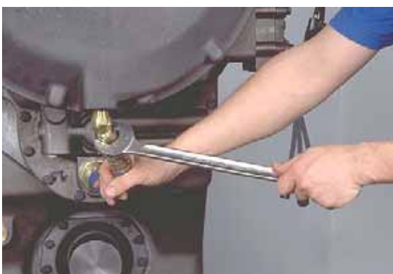
Figure 3 Remove drain hose from front cover as shown.
