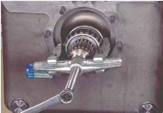
Figure 55 Remove output shaft rear bearing cone.
