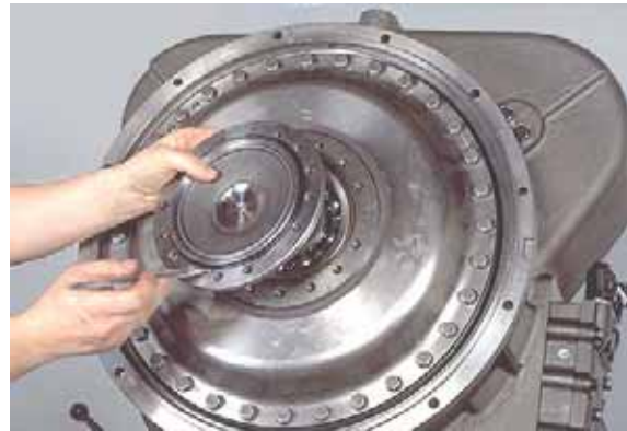
Figure 4 Remove impeller cover bearing cap and "O"-ring.
