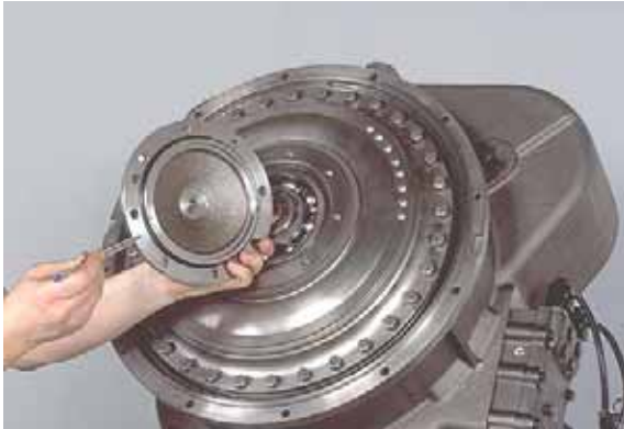
Figure 9 Position new "O"-ring on input shaft.
