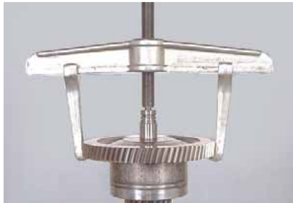
Figure 157 Remove low clutch gear and outer bearing.
