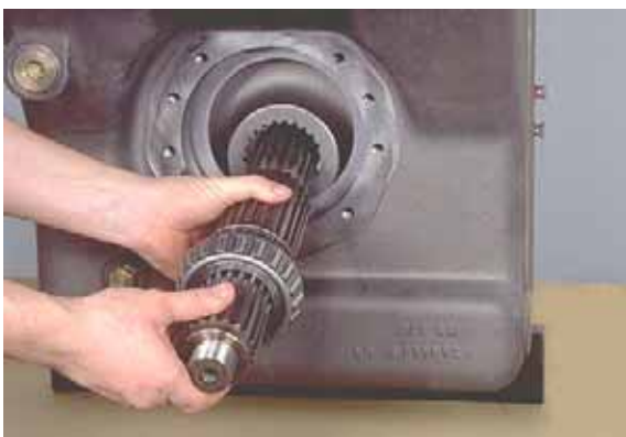
Figure 57 From the front side. Remove output shaft and bearing cone as an assembly.
