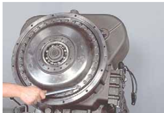
Figure 6 Remove impeller to impeller cover mounting screws.
