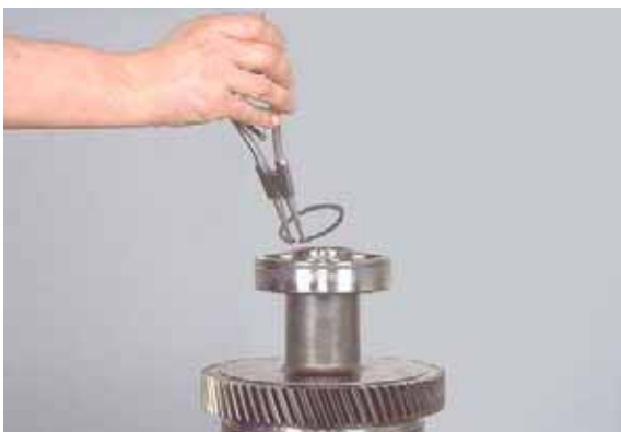
Figure 132 Remove clutch shaft rear bearing retaining ring.
