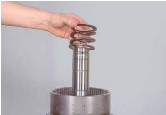
Figure 130 Remove piston return spring.
