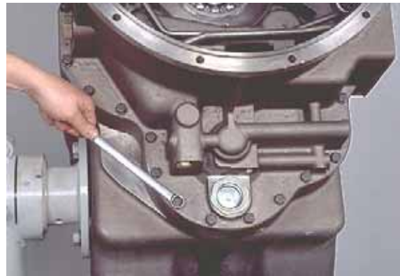
Figure 23 Support converter housing with a chain hoist and strap. Remove converter housing to transmission housing screws and lockwashers.
