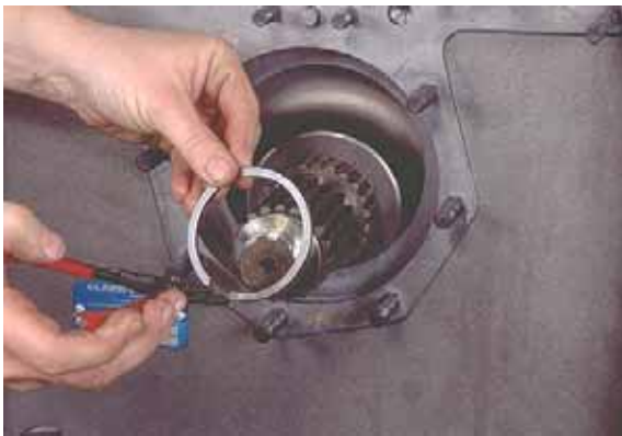
Figure 56 Remove output shaft gear retaining ring.
