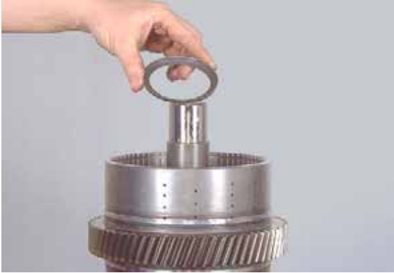
Figure 91 Remove spring retainer.
