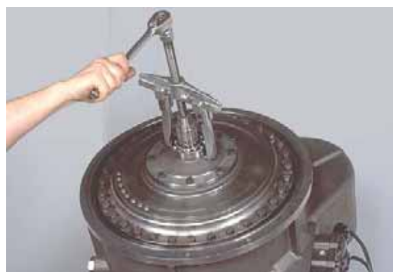
Figure 6 Remove input shaft support bearing.
