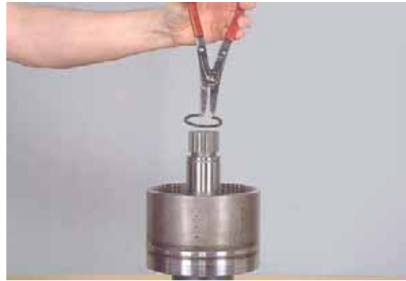
Figure 196 Remove inner bearing locating ring.
