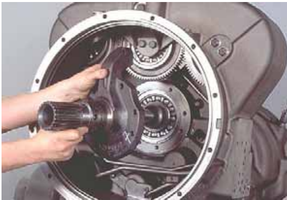
Figure 20 Turn support to clear drive gear. Remove stator support.
