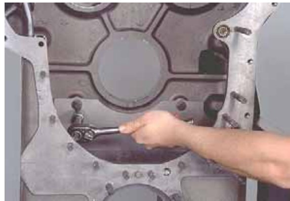
Figure 59 Remove oil baffle mounting screws and lockwashers.
