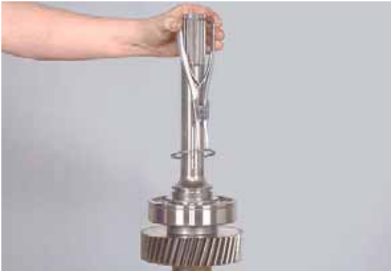
Figure 252 Remove turbine shaft front bearing retaining ring.
