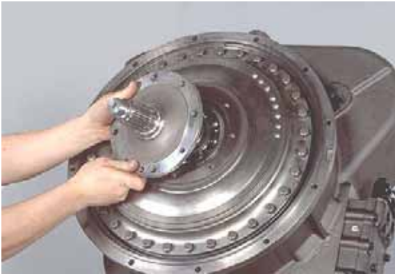
Figure 8 Input shaft removed.
