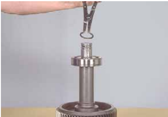
Figure 219 Remove 4th shaft front bearing retaining ring.
