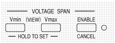
V-Span is turned on or off with the ENABLE key. The ENABLE lamp is lit when V-Span is selected. The factory default is  $V_{\min} = 3V$ ,  $V_{\max} = 5V$
