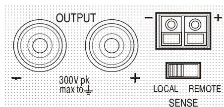
This problem can be minimised by using short, thick, connecting leads, but where necessary it can be completely overcome by using the remote sense facility.
