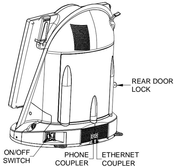
FIGURE 33 - REAR VIEW OF THE IONAURORA
