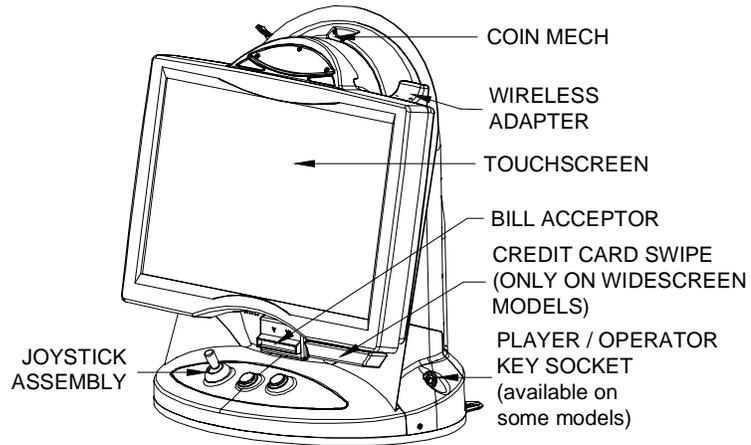
FIGURE 32 - FRONT VIEW OF THE IONAURORA
