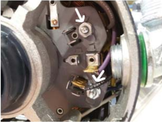
Showing connection points in 1 HP, 120v motor black & white wires attach to spades left of two nuts
