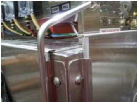
Showing misaligned arms on corner
