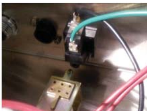
Optional Chemical Alarm switch, buzzer
