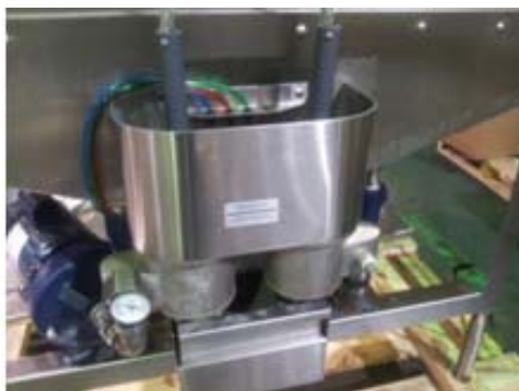
5AGES sump, drain ball, water level decal, chemical tubes, scrap box
