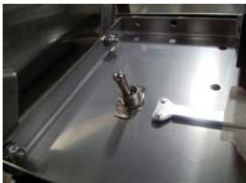
De-lime switch in control box
