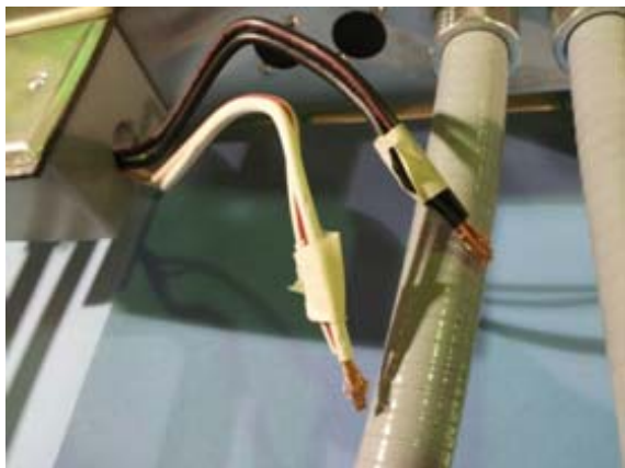
Showing single circuit wire combination
