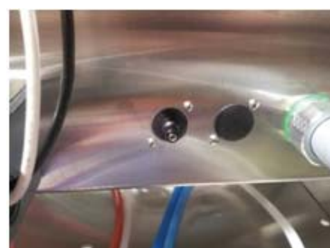
Chemical alarm barb adjusting screw *
