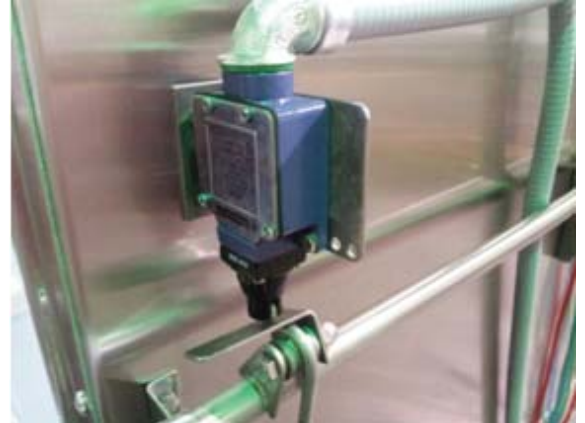
5AGES Door cut-off switch and lever arm
