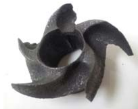
Impeller damaged from high acid solution
