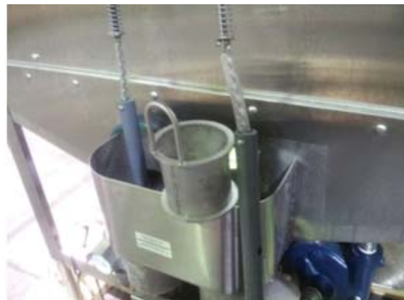
5AGES sump, drain balls and stainless filters
