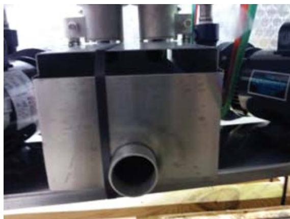
Showing scrap box as installed on 5AGES or WS2
