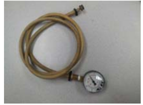
Spray arm pressure tester #088-1048
